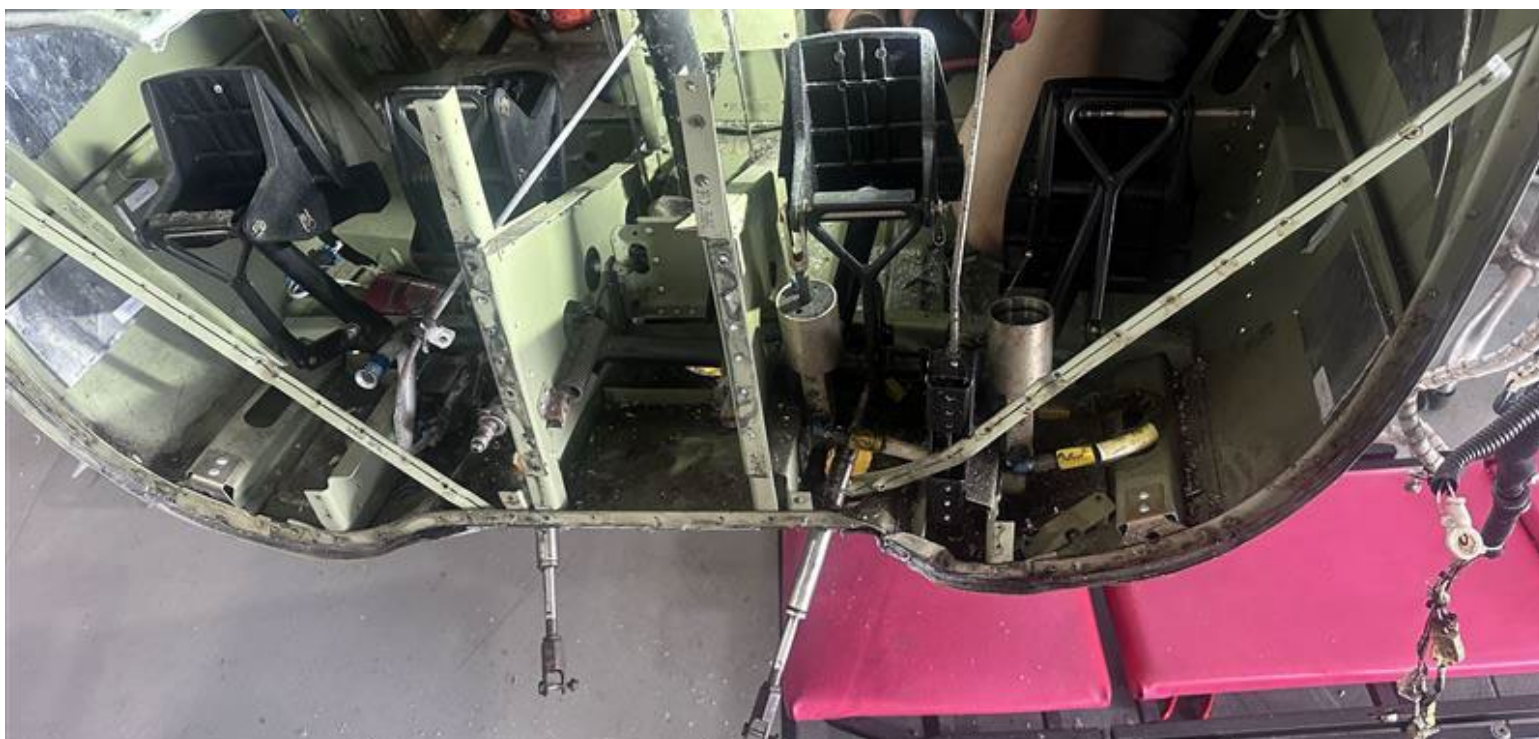
Photograph 3 - Lower fuselage impact damage (Courtesy of Flight School)
