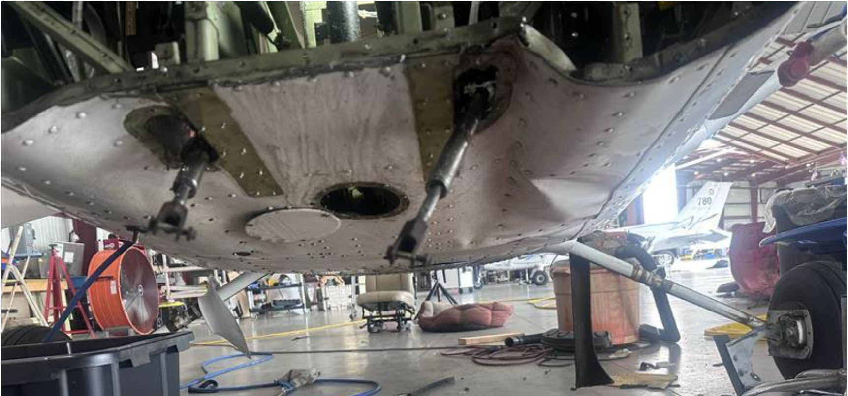
Photograph 1 - Lower fuselage impact damage (Courtesy of Flight School)
