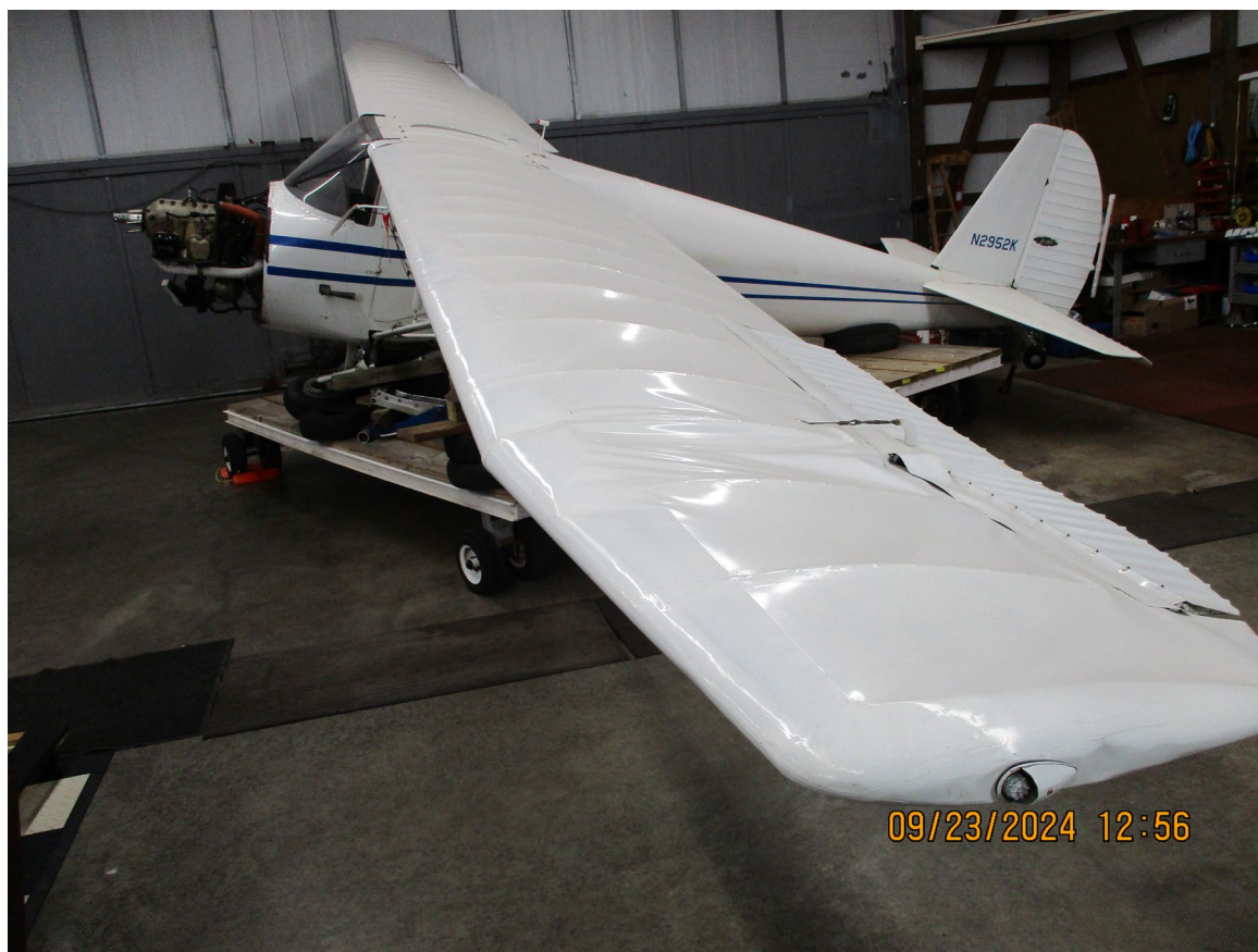
Photograph 2 - Damage to the Left Wing (Courtesy of FAA)
