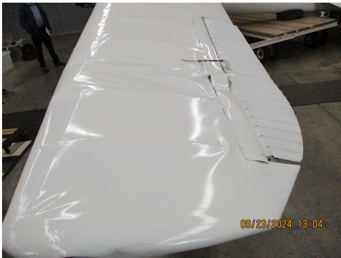
Photograph 3 - Damage to the Left Wing (Courtesy of FAA)
