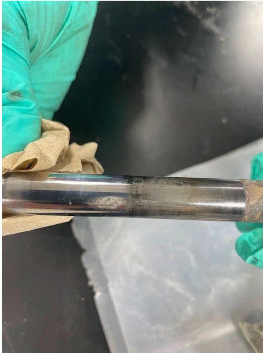
Photograph 11 - No. 3 Exhaust Valve Stem at Lycoming Materials Exam (NTSB Photo)
