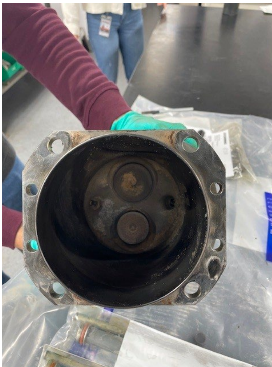
Photograph 8 - No. 3 Cylinder Bore at Lycoming Materials Exam (NTSB Photo)
