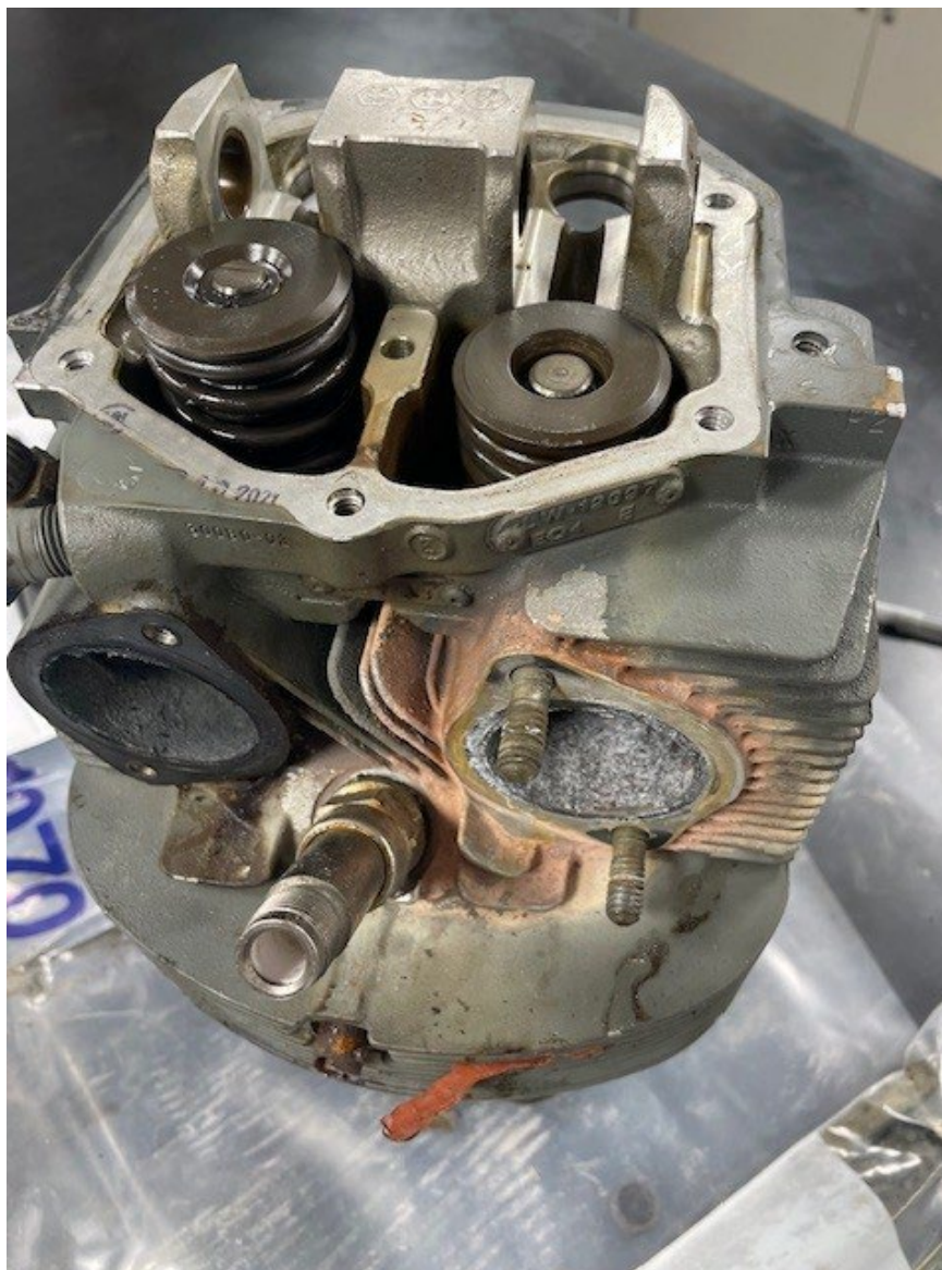
Photograph 9 - No. 3 Cylinder at Lycoming Materials Exam (NTSB Photo)
