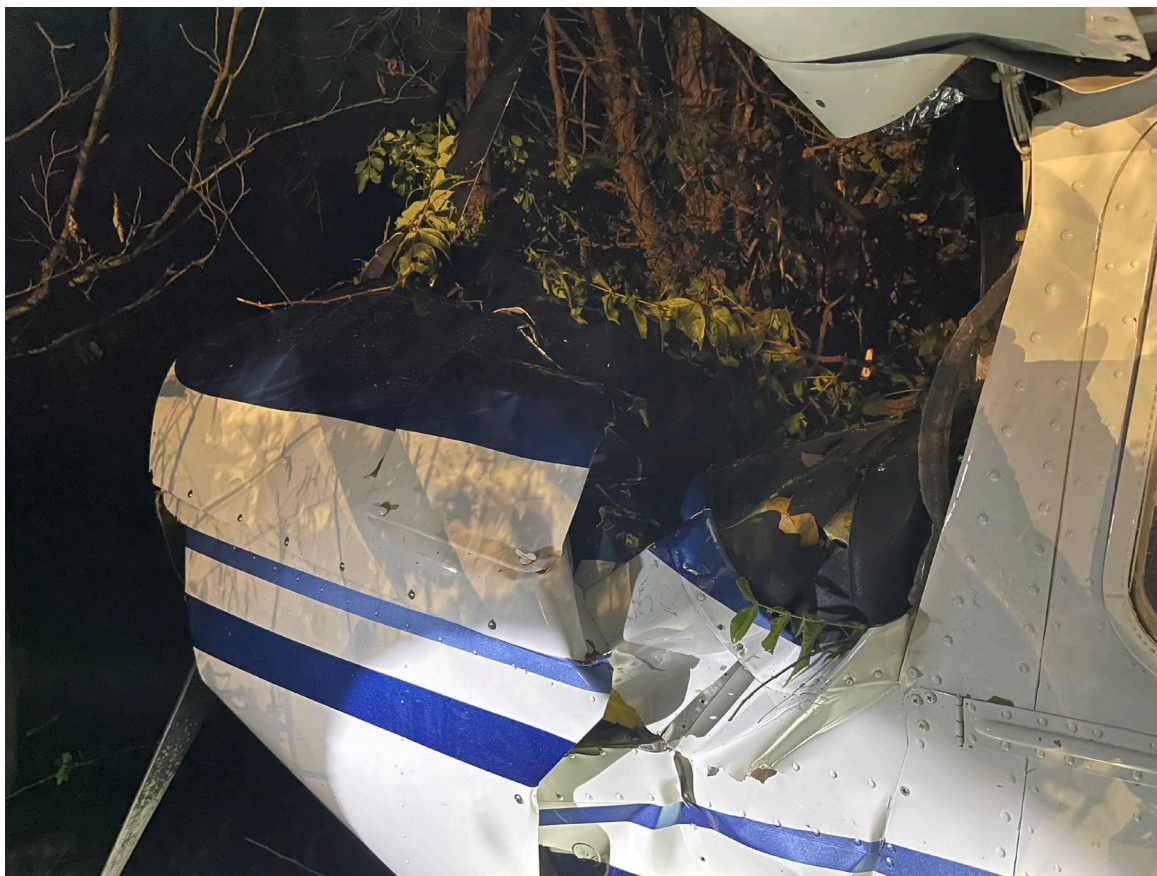
Photograph 2 – View of crushed engine cowling and fuselage (Courtesy of FAA)
