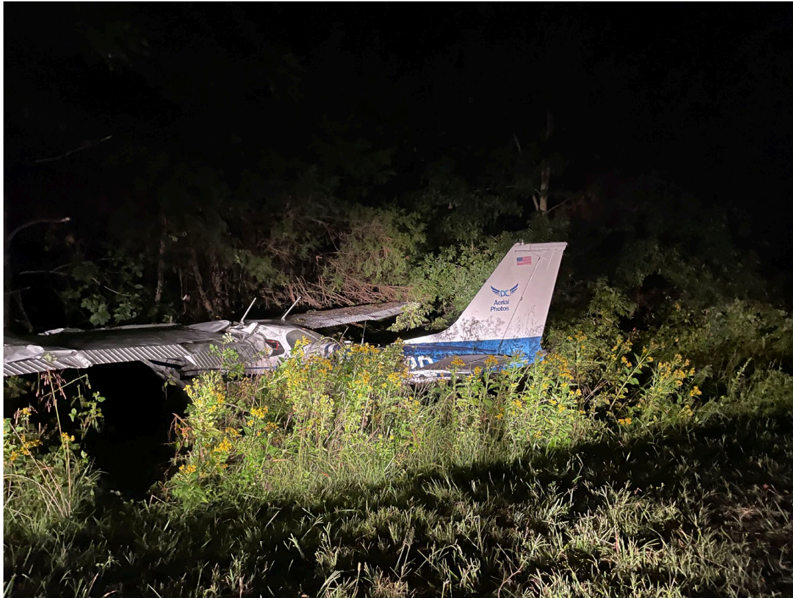
Photograph 1 –View of airplane in wooded area showing damaged left wing. (Courtesy of FAA)
