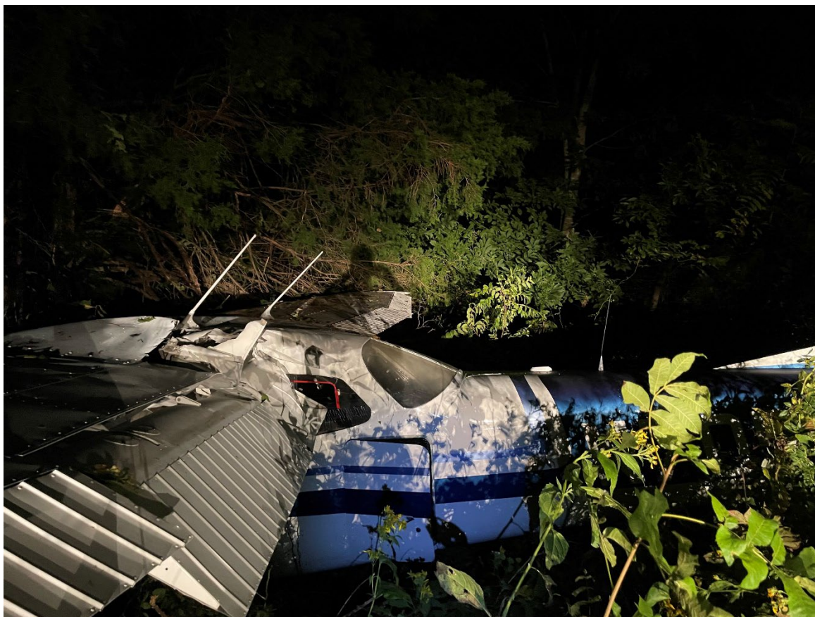
Photograph 3 –View of buckled left wing root and upper fuselage damage. (Courtesy of FAA)
