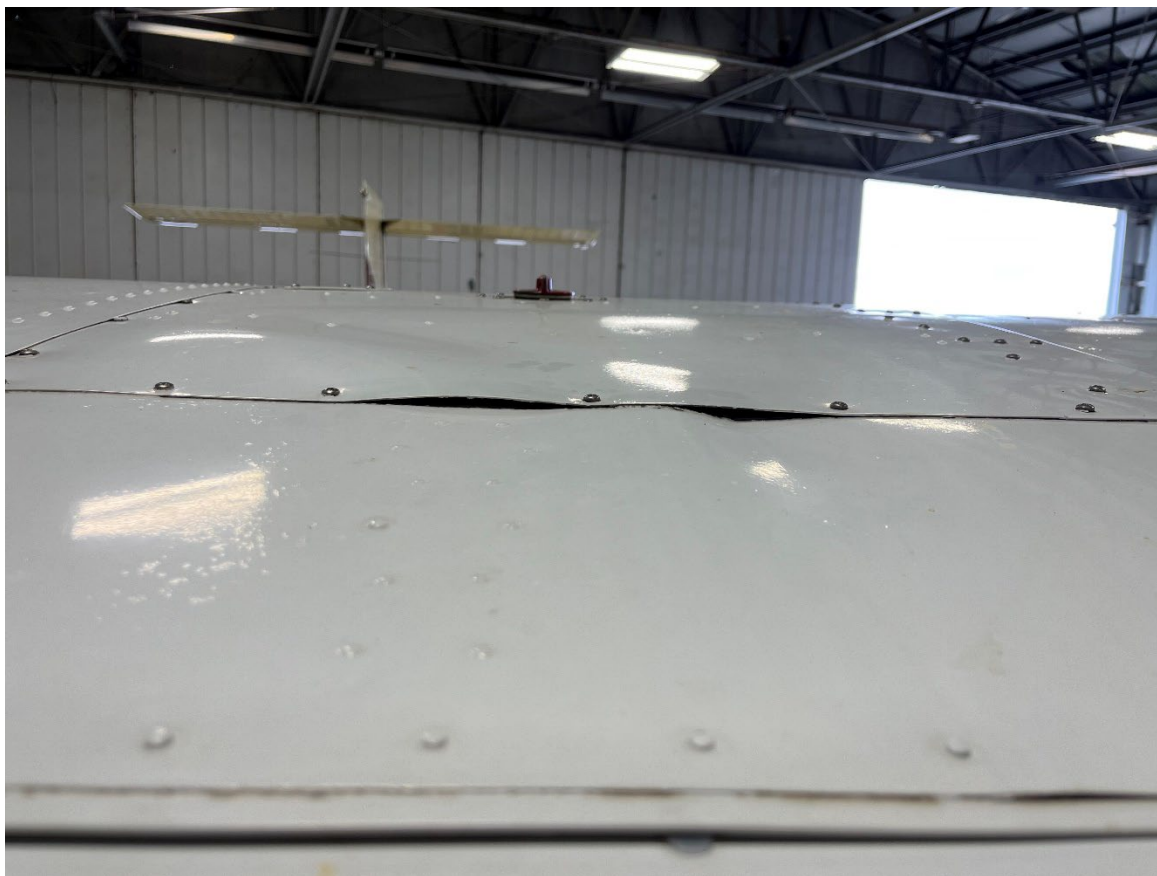
Photograph 3 - Right wing impact damage buckling(Courtesy of FAA)
