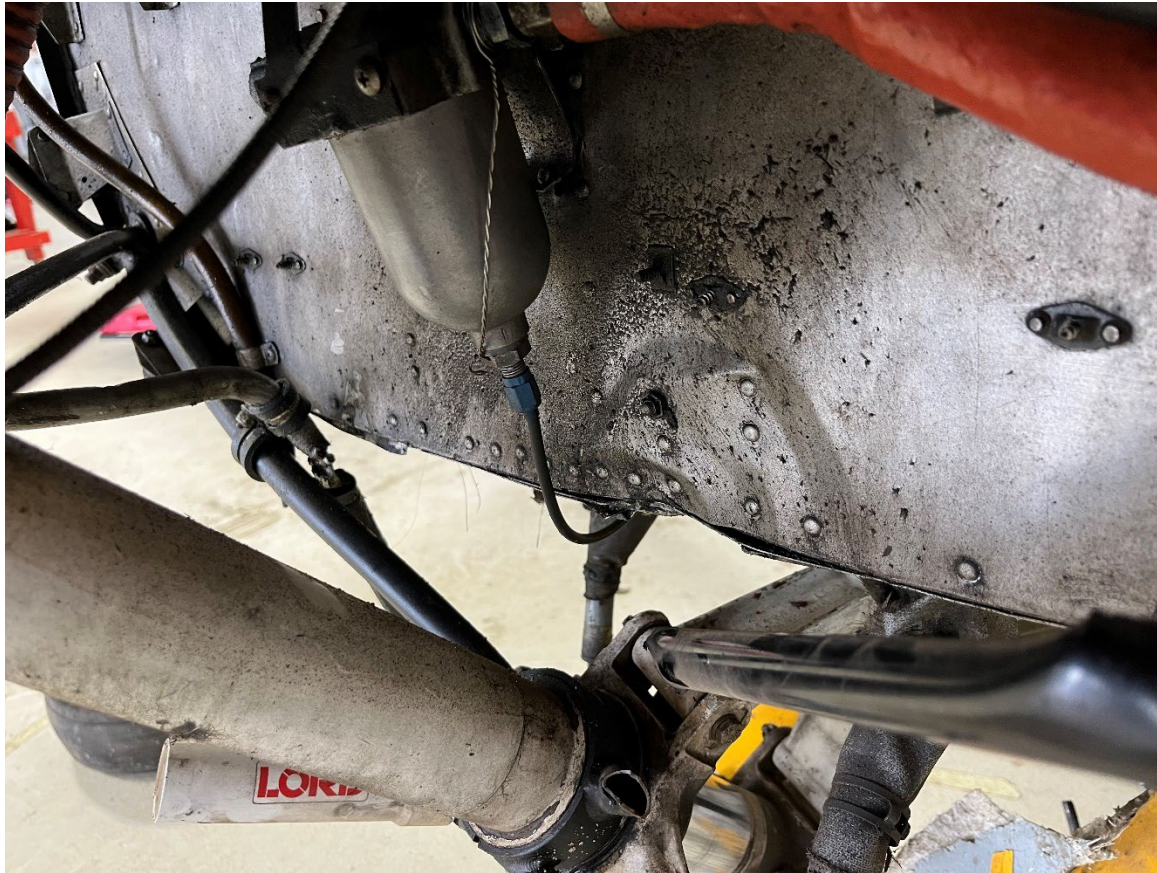
Photograph 3 - Lower fuselage impact damage (Courtesy of FAA)
