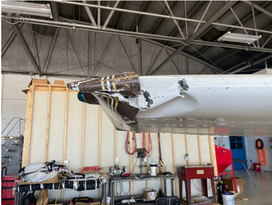
Photograph 2 - Right wing impact damage (Courtesy of FAA)
