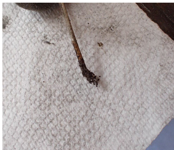
Photograph of debris recovered from the rear oil passage of the crankcase's front main bearing area.
