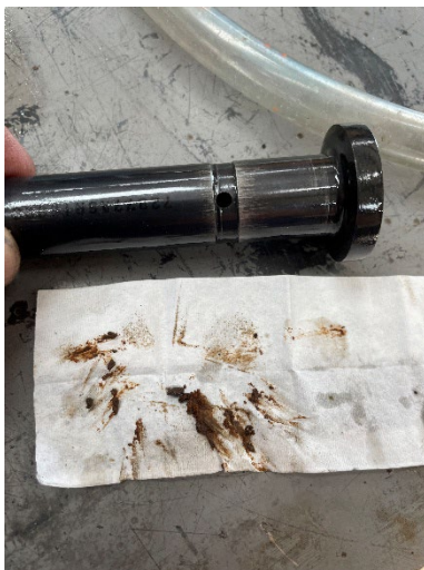
Photograph of the No. 4 cylinder intake cam follower and oil passage debris.
