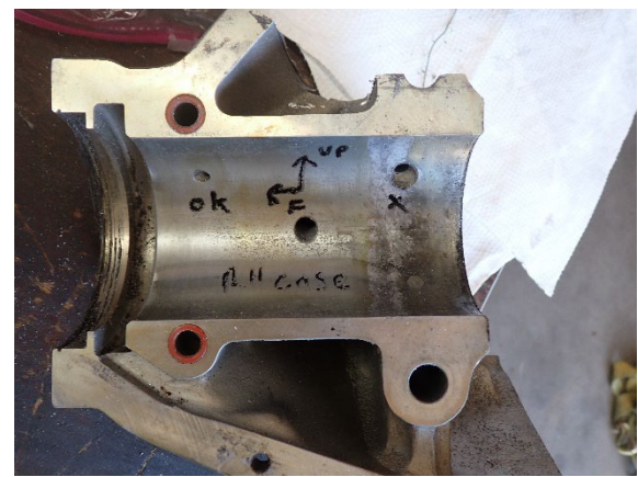
Photograph of sectioned crankcase and noted obstructed passage.
