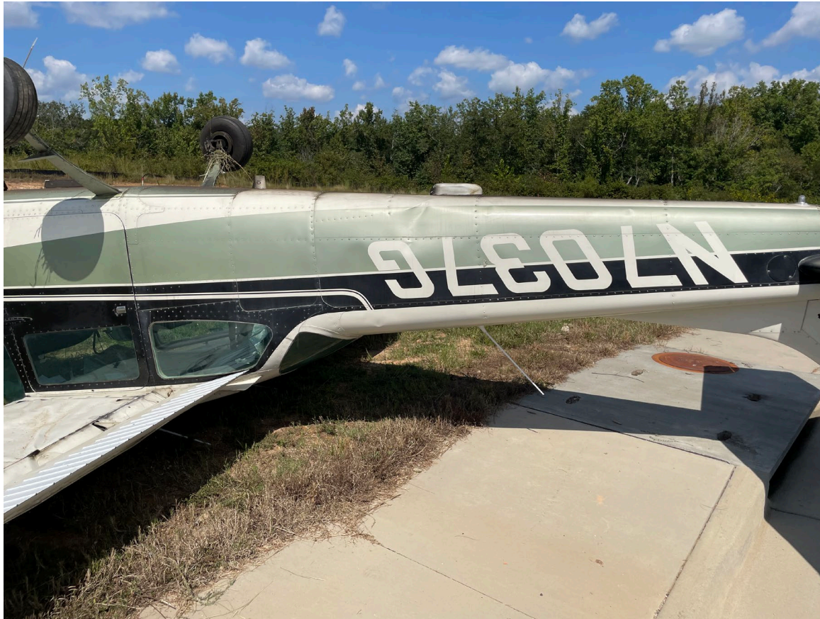
Photograph 3 - Buckling noted to fuselage (Courtesy of FAA)
