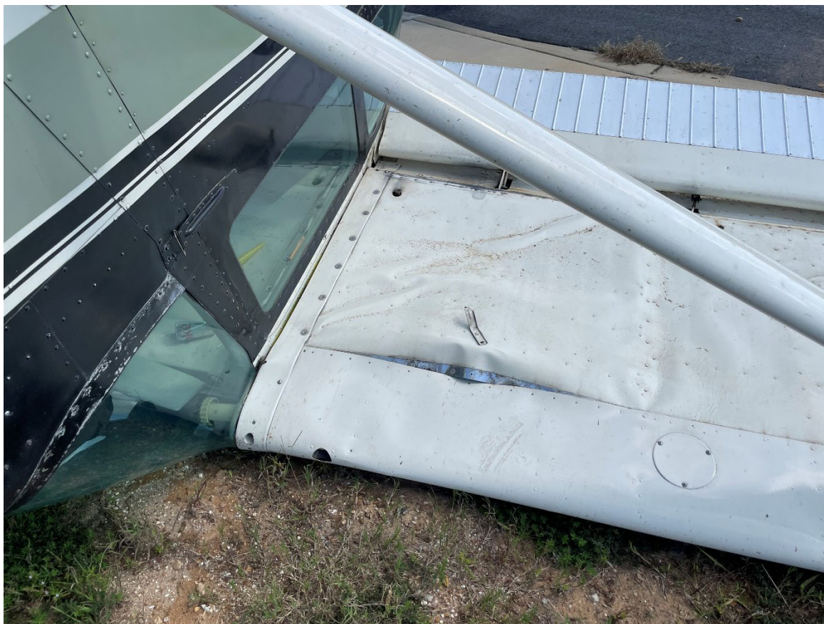
Photograph 2 - Deformation and skin separation noted to right wing (Courtesy of FAA)
