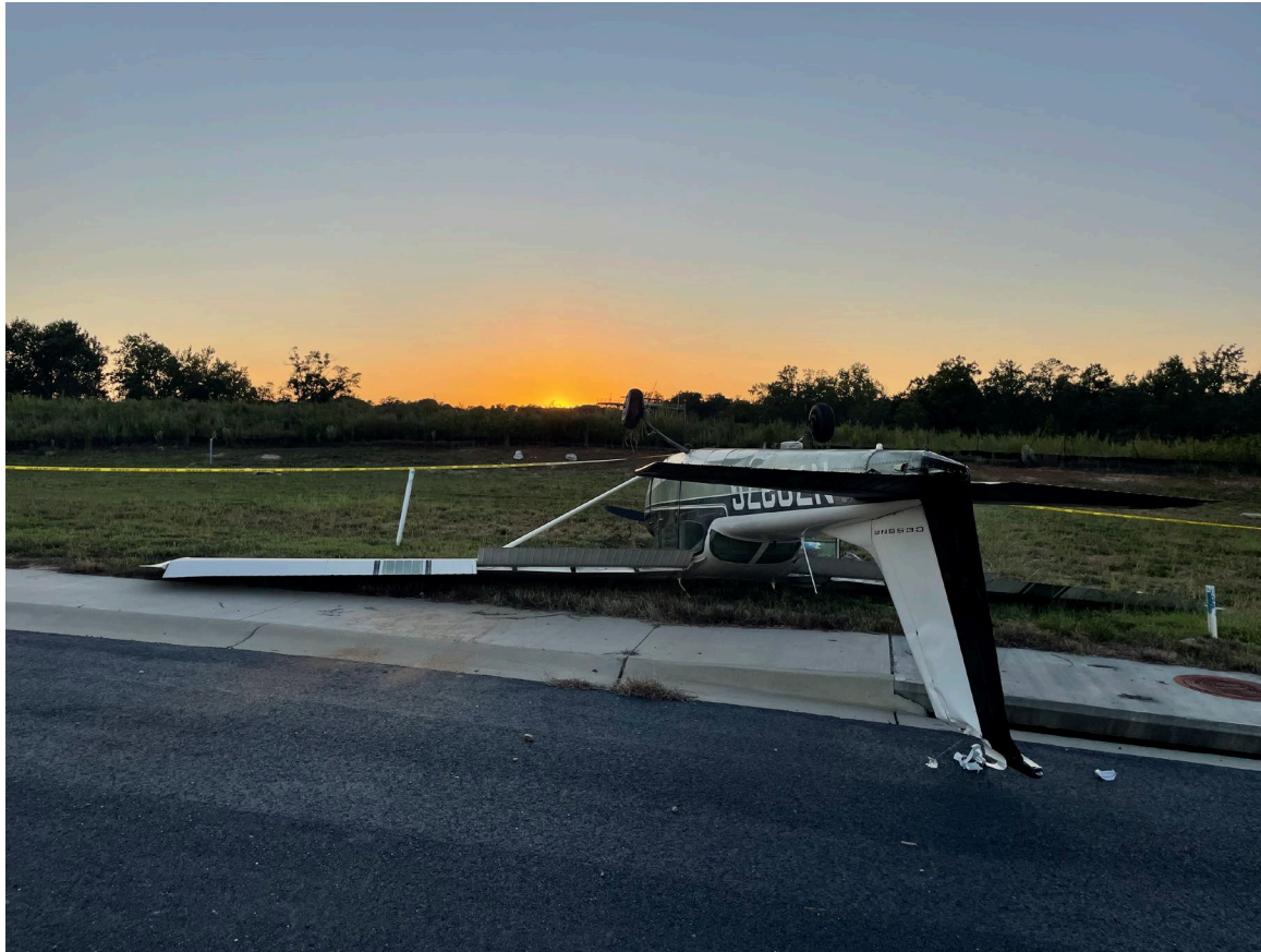
Photograph 1 - Deformation noted to rudder and vertical stabilizer (Courtesy of FAA)
