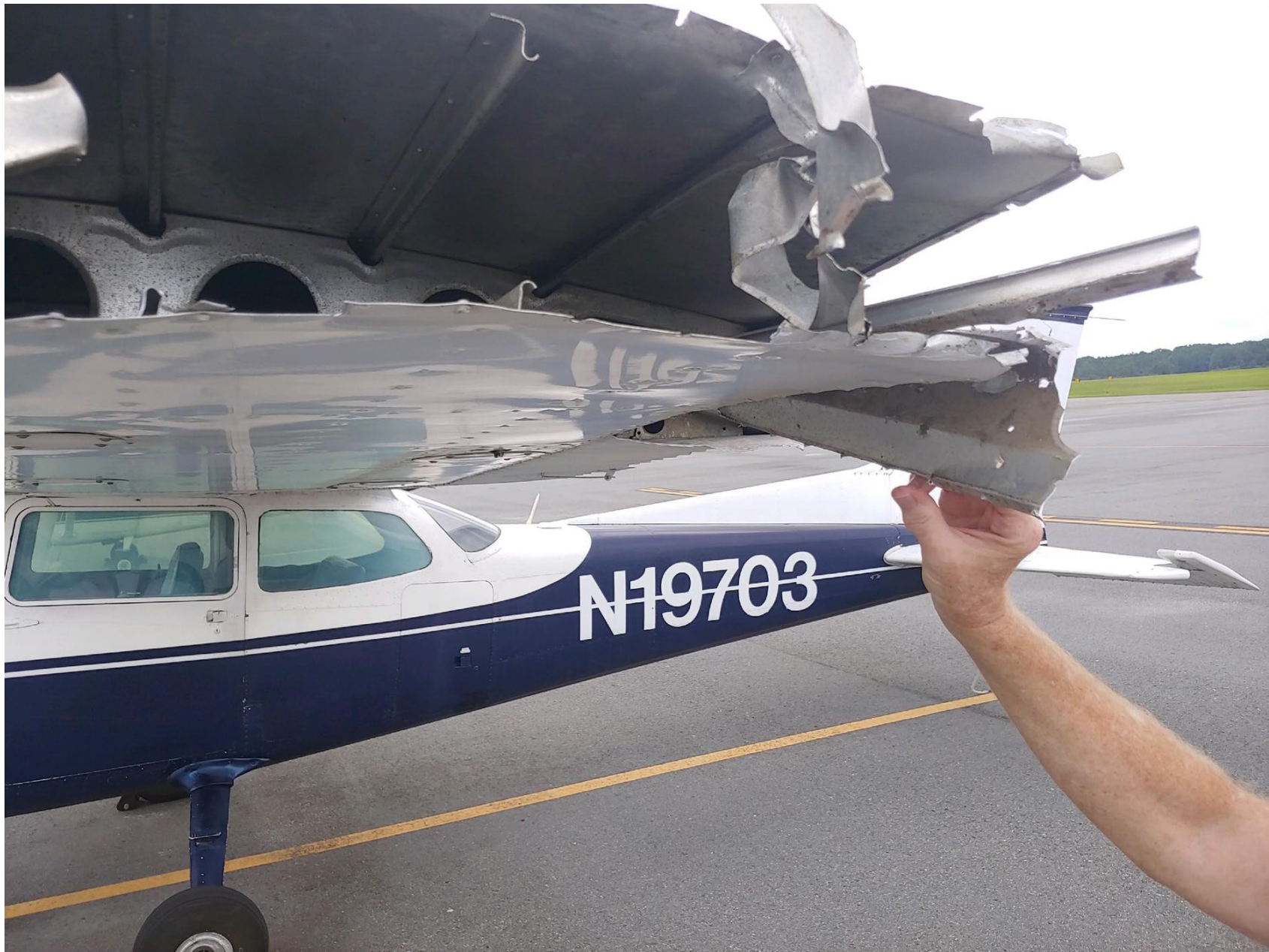
Photo 2 – View of Wing Trailing Edge Damage (FAA)
