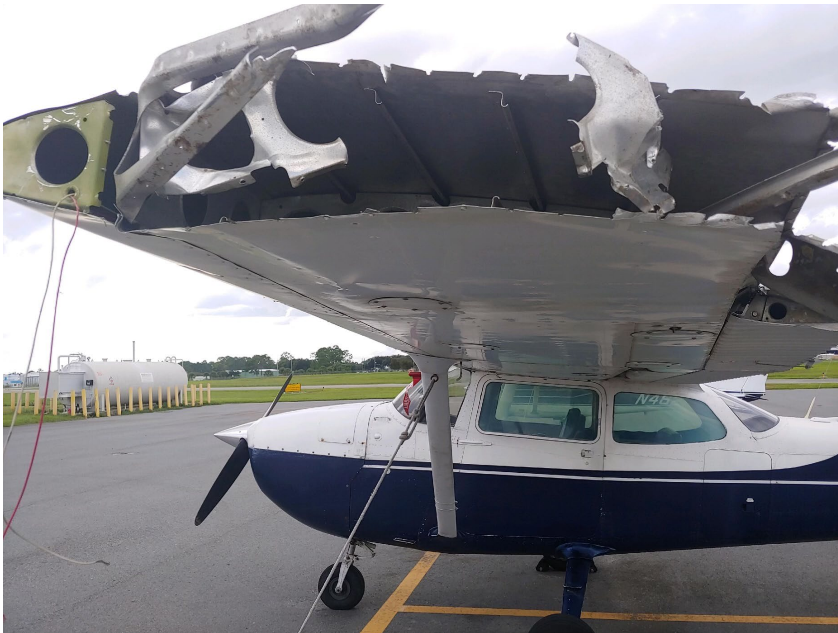
Photo 1 – View of Wingtip Damage (FAA)
