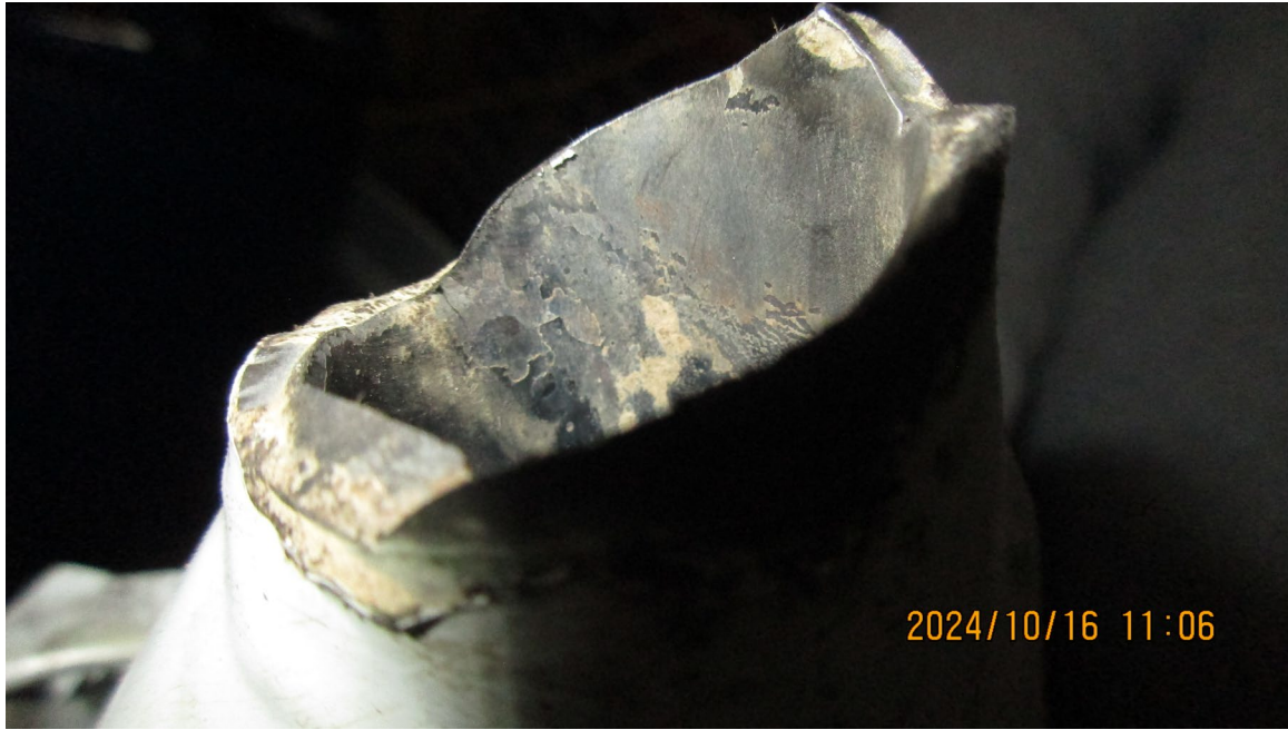
Photograph 5 - Close up of left landing gear strut assembly fracture edges. (Courtesy of FAA)
