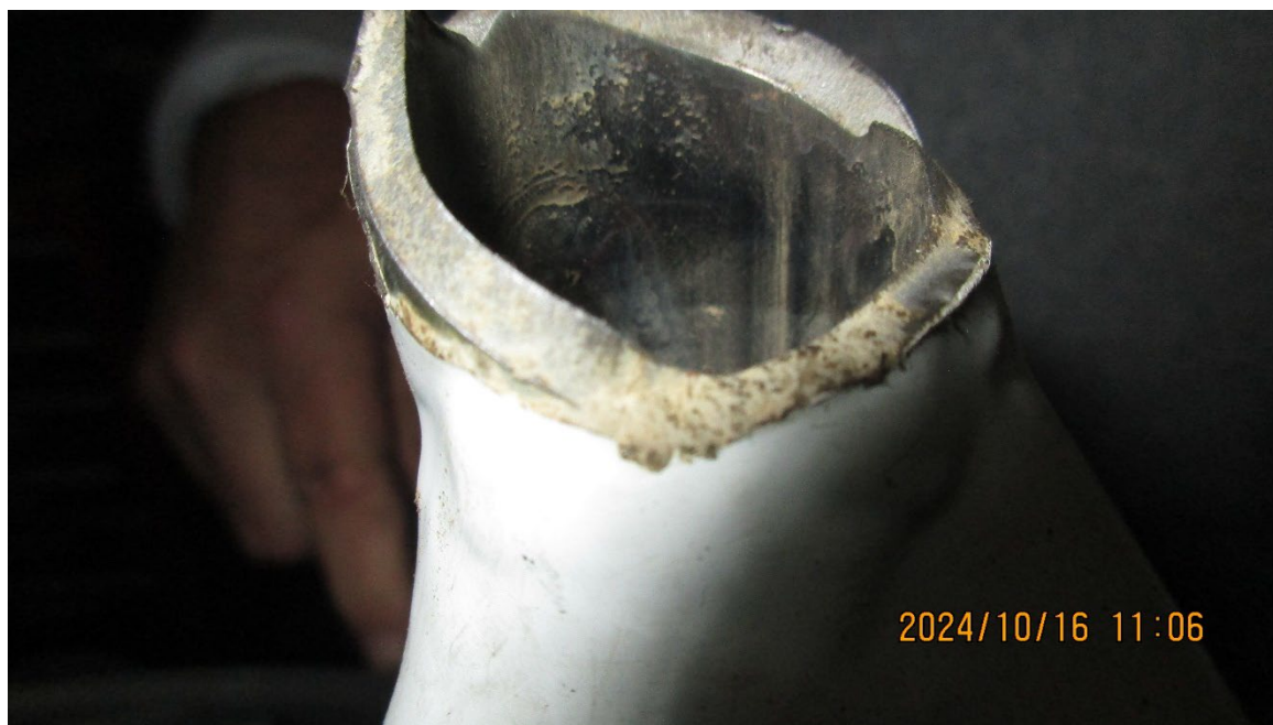
Photograph 4 - Close up of left landing gear strut assembly (side view) fracture. (Courtesy of FAA)
