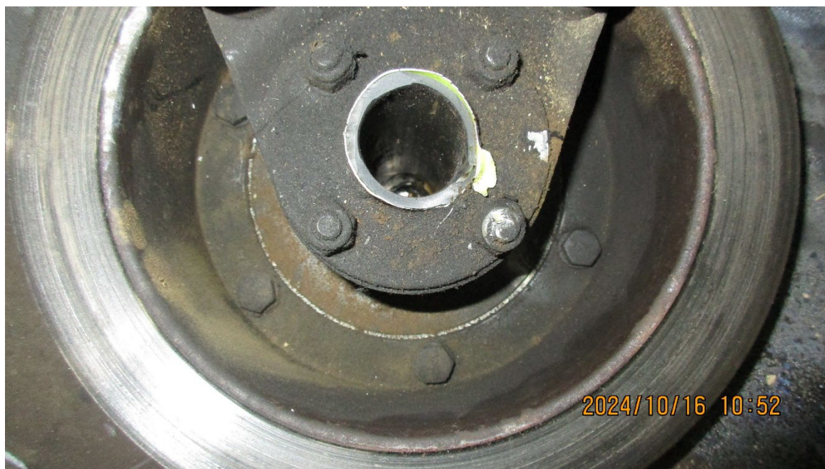
Photograph 6 - Close up of fractured wheel assembly. (Courtesy of FAA)
