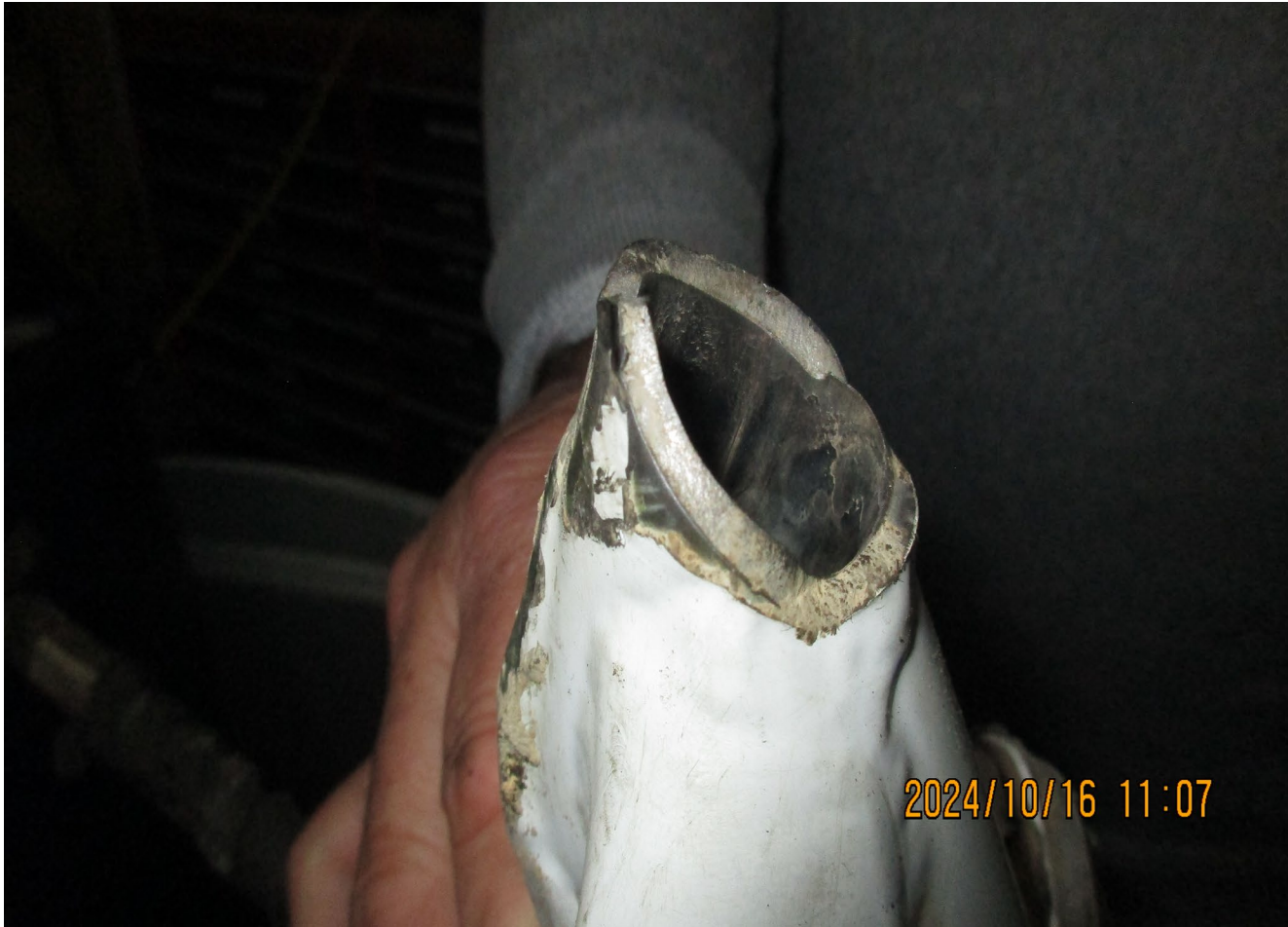
Photograph 2 - View of broken left landing gear strut (Courtesy of FAA)
