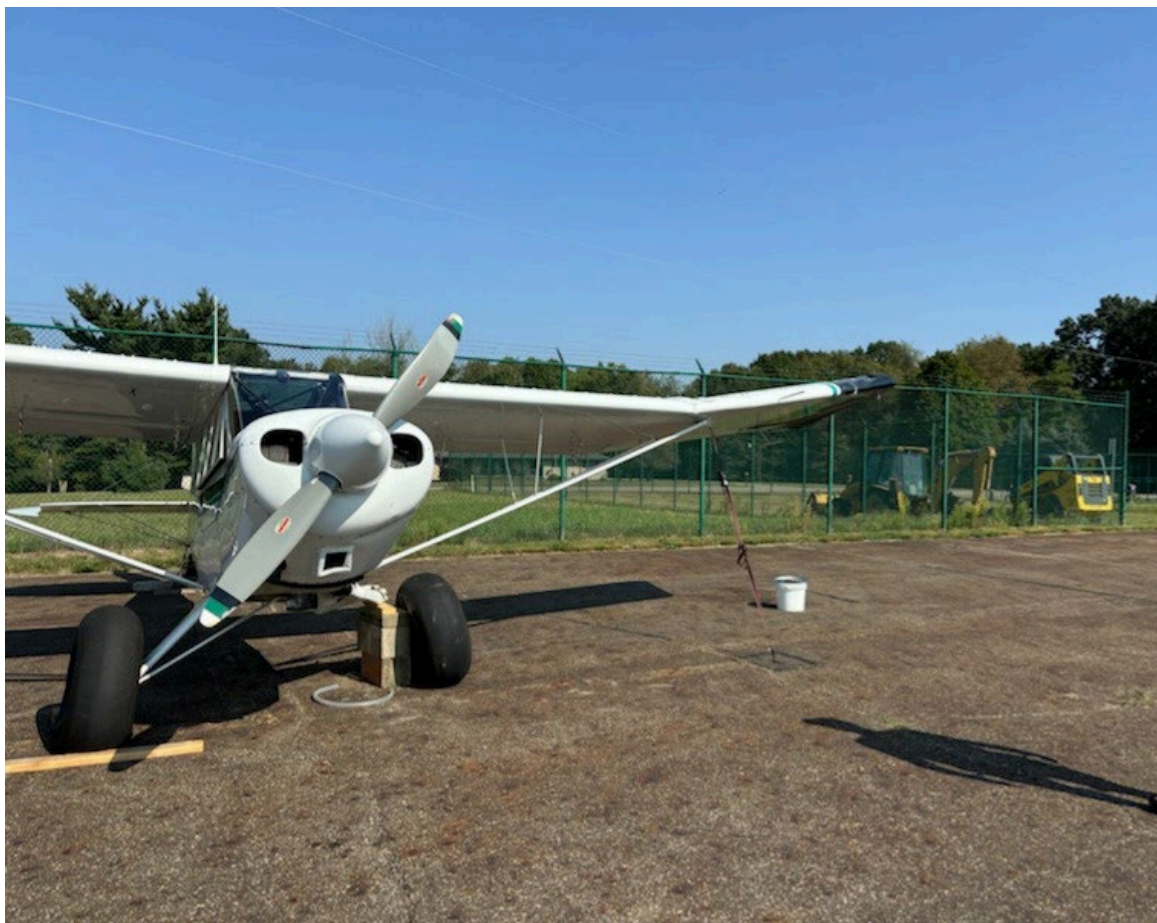
Photograph 1 - View of blue and white airplane with left wing bent upwards. (Courtesy of FAA)
