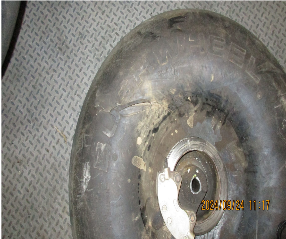
Photograph 3 - View of broken landing gear wheel assembly (Courtesy of FAA)
