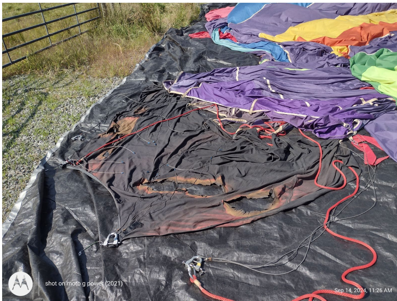
Photograph 2 - Damaged balloon and cables. (Courtesy of Pilot/Owner)
