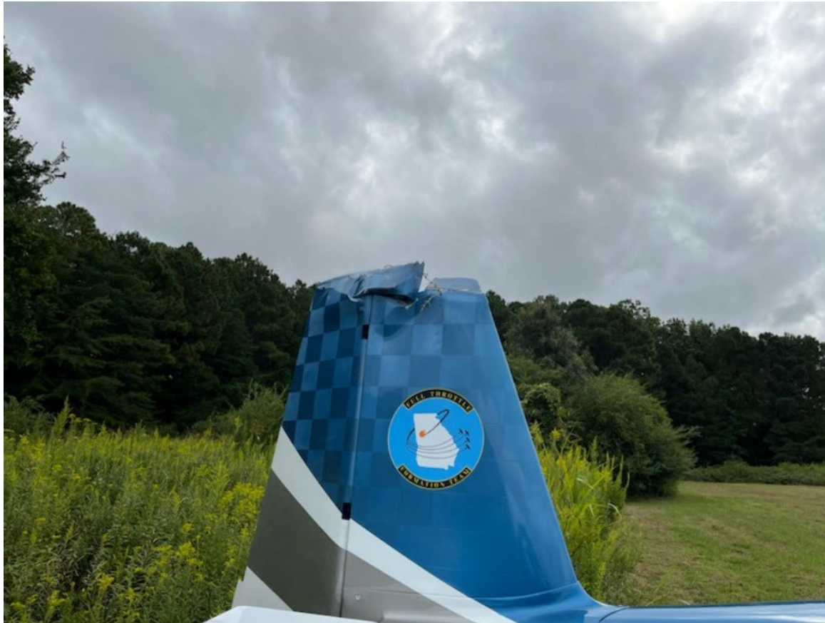
Photograph 3 - Damage to Vertical Stabilizer and Rudder (Courtesy of FAA)
