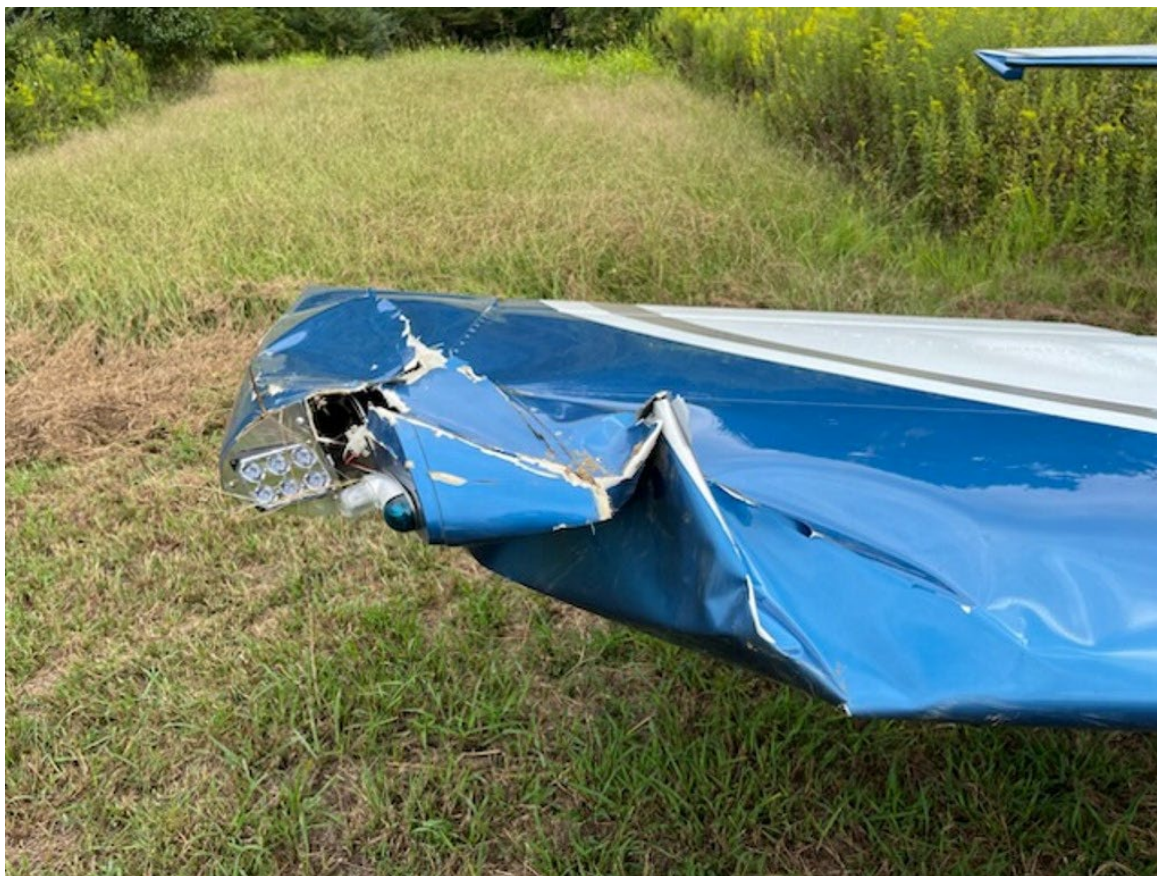
Photograph 2 - Damage to Right Wing (Courtesy of FAA)
