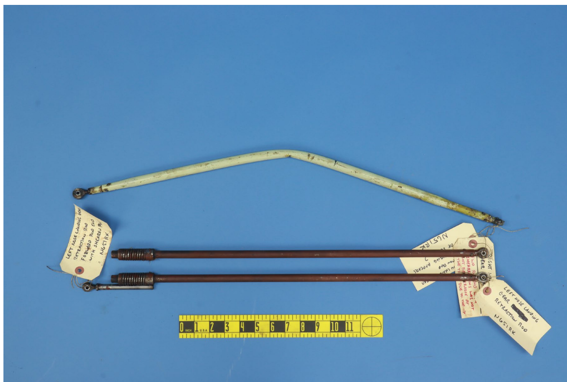
Photograph 6 - Bent Right Main Landing Gear Extension Rod and Nose Gear Extension Rods (NTSB Photo)
