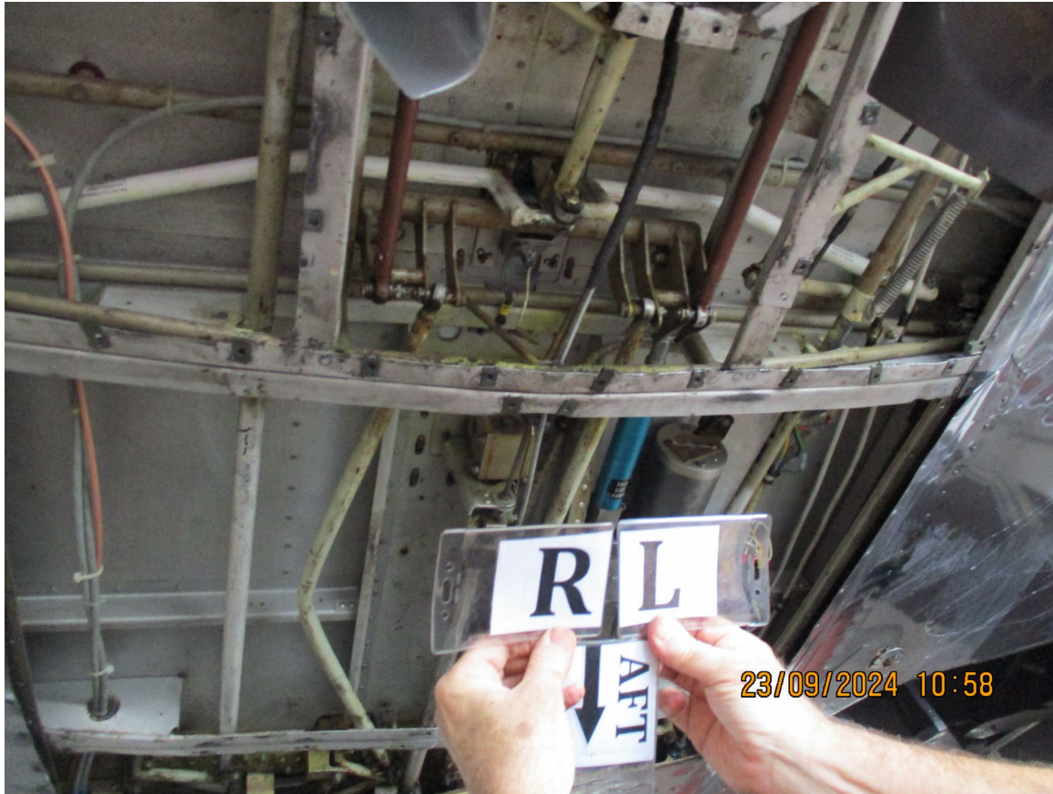
Photograph 5 - Bent Right Main Landing Gear Extension Rod (FAA Photo)
