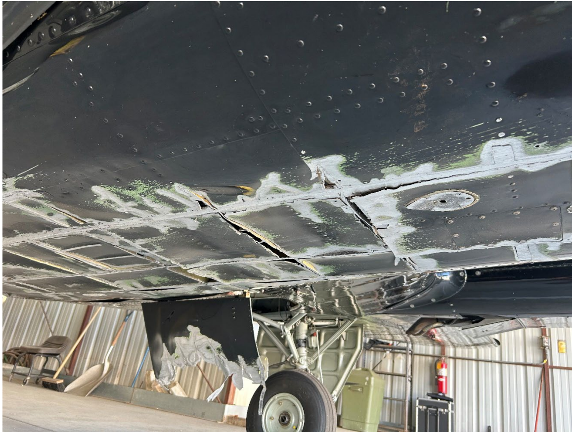
Photograph 3 - Lower fuselage accident damage (Courtesy of FAA)
