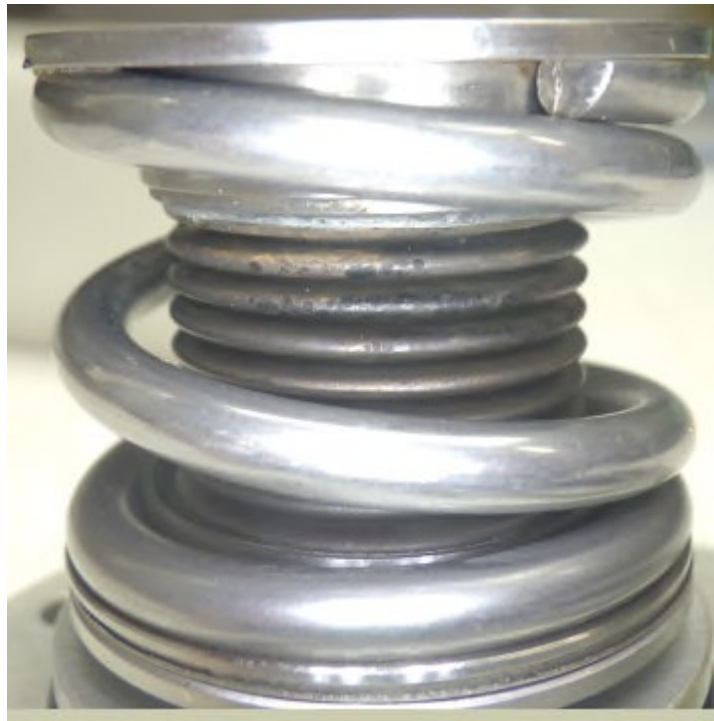
Figure 3: Bellows with contamination. (Courtesy of P&WC)
