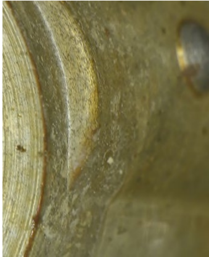
Figure 5: Bellows housing cavity contamination. (Courtesy of P&WC)
