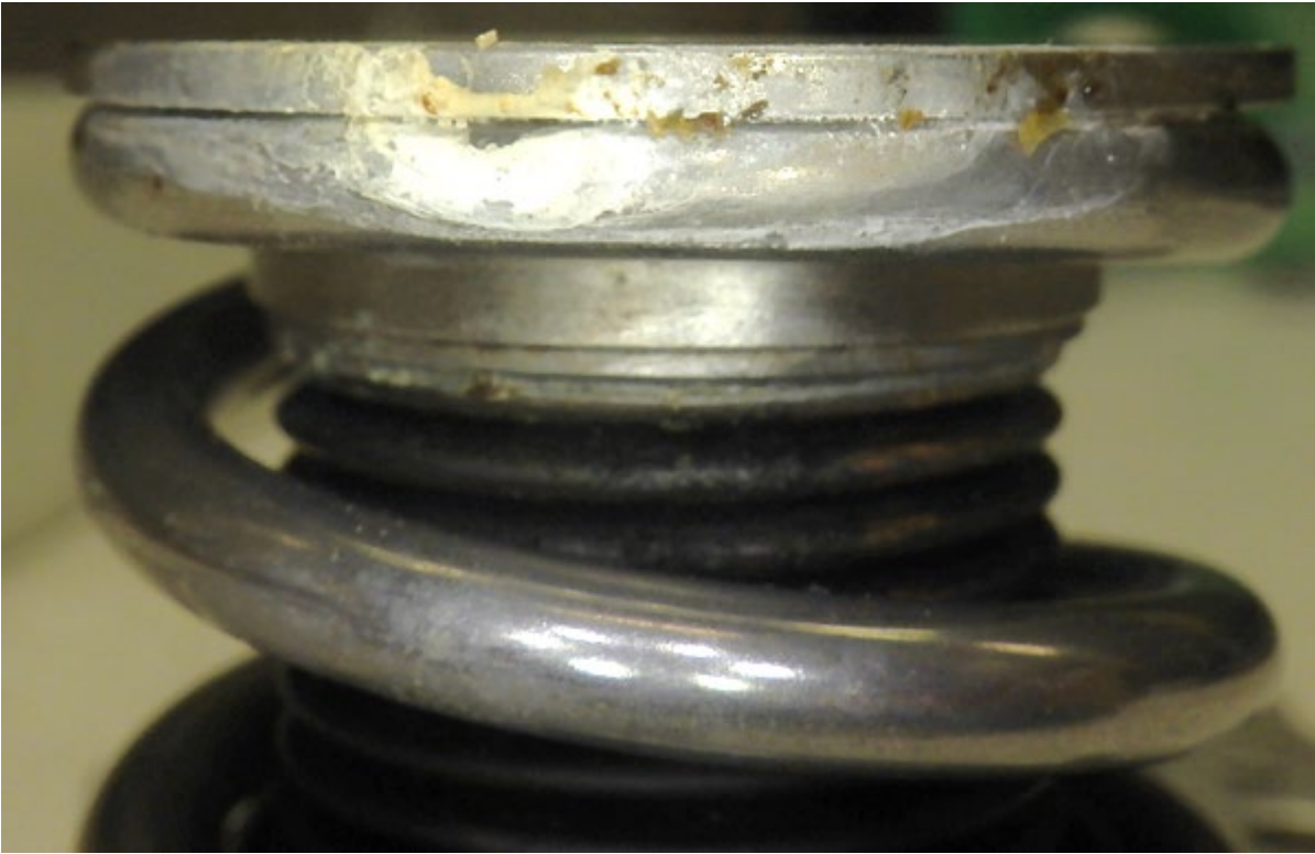
Figure 4: Bellows contamination. (Courtesy of P&WC)
