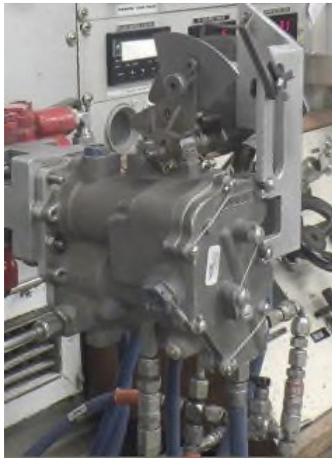
Figure 2: FCU installed on the test stand. (Courtesy of P&WC)
