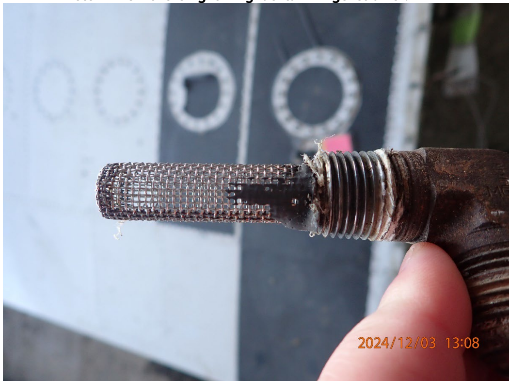
Photo 3: View of the left wing fuel tank finger strainer.
