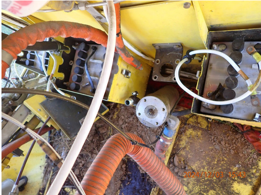
Photo 4: View of the fuel strainer after being removed from the mounting bracket.
