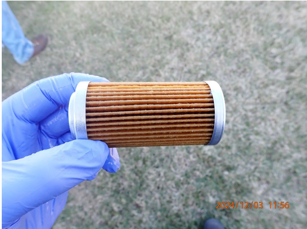
Photo 8: View of the fuel control unit fuel filter.
