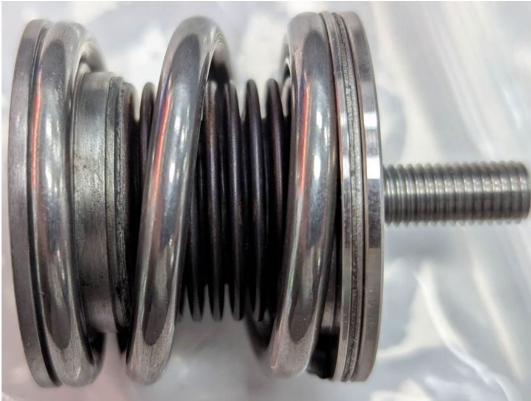
Figure 4: View of the cleaned bellows. (Courtesy of Woodward)
