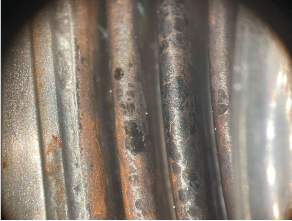
Figure 2: View of corrosion on the bellows assembly. (Courtesy of Woodward)
