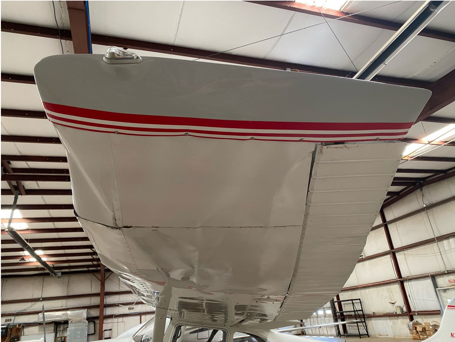
Photograph 2 - left wing tip bent up (Courtesy of the owner)
