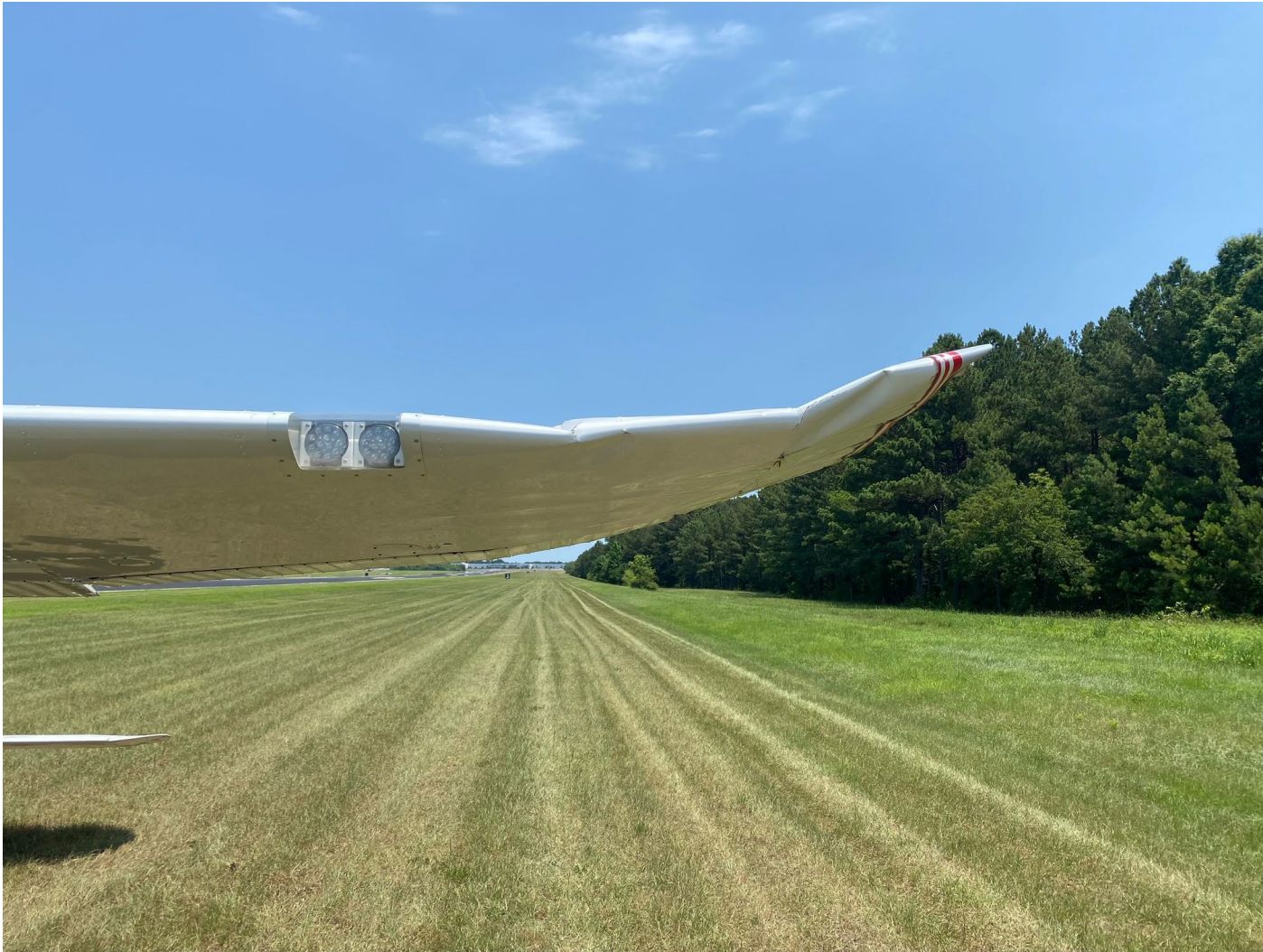
Photograph 1 - left wing tip bent up (Courtesy of owner)
