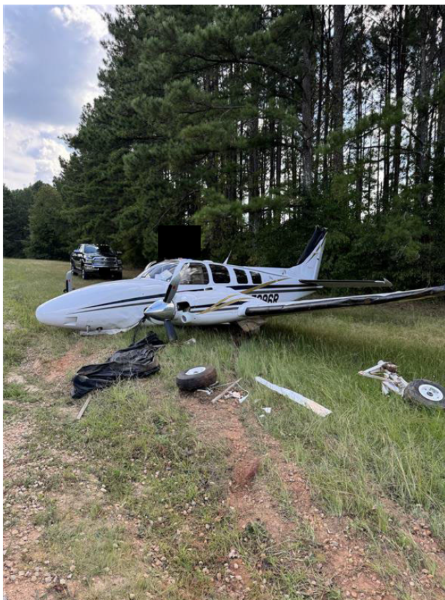
Photograph 2 - Forward Fuselage Damage (Courtesy of FAA)
