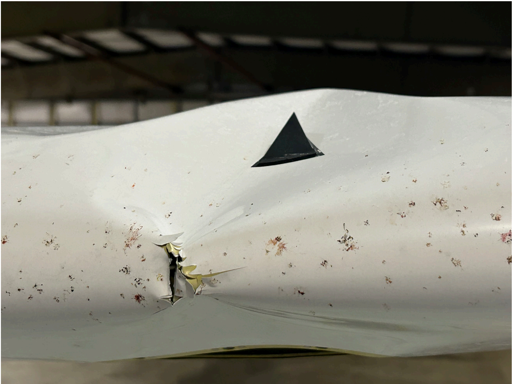
Photo 3 – View of Left Wing Leading Edge Damage (FAA)
