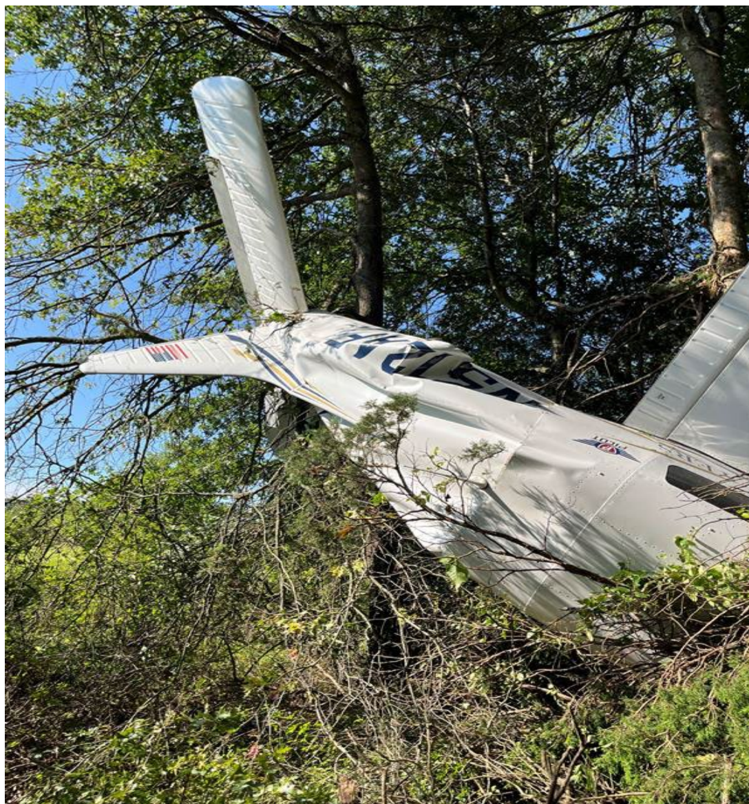
Photograph 2 - Buckled fuselage resting against a tree. (Courtesy of FAA)
