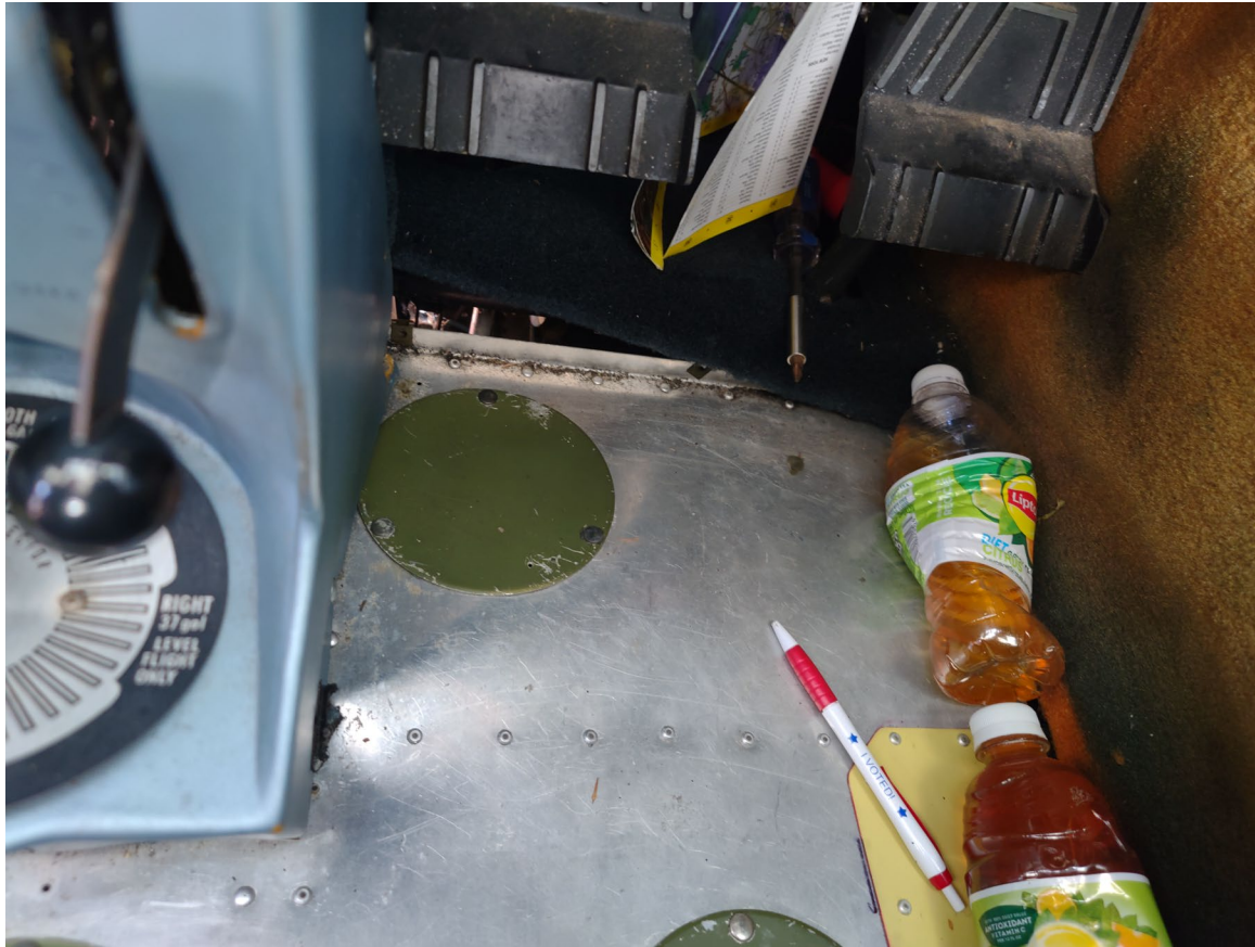
Photograph 2 - Deformation noted to the lower forward fuselage structure (Courtesy of FAA)
