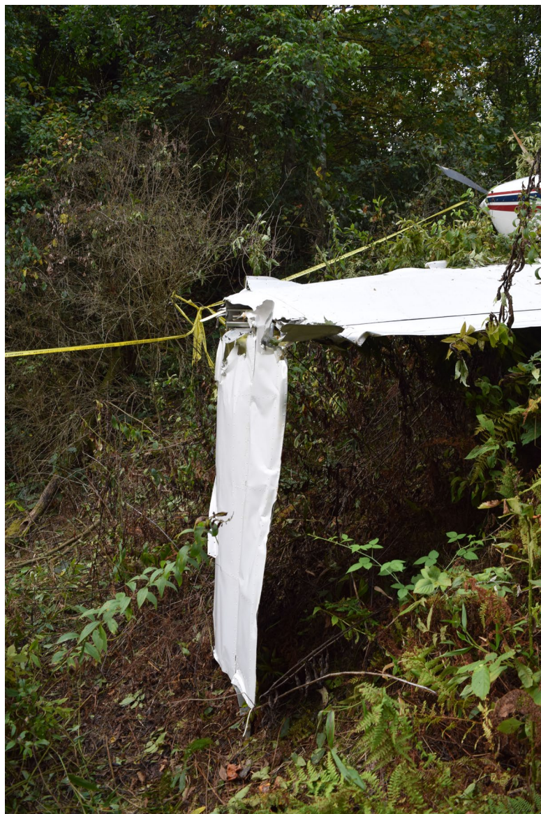
Photograph 4 - FAA Digital Photograph. View of the Nearly Completely Fractured Left Wing
