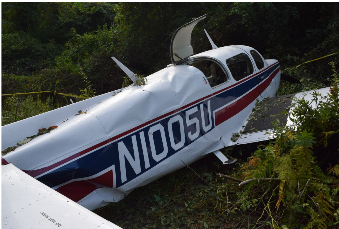
Photograph 3 - FAA Digital Photograph. Right Rear Quartering View of the Airplane At the Accident Site. Note the Compression Wrinkles in the Right Side of the Aft Fuselage
