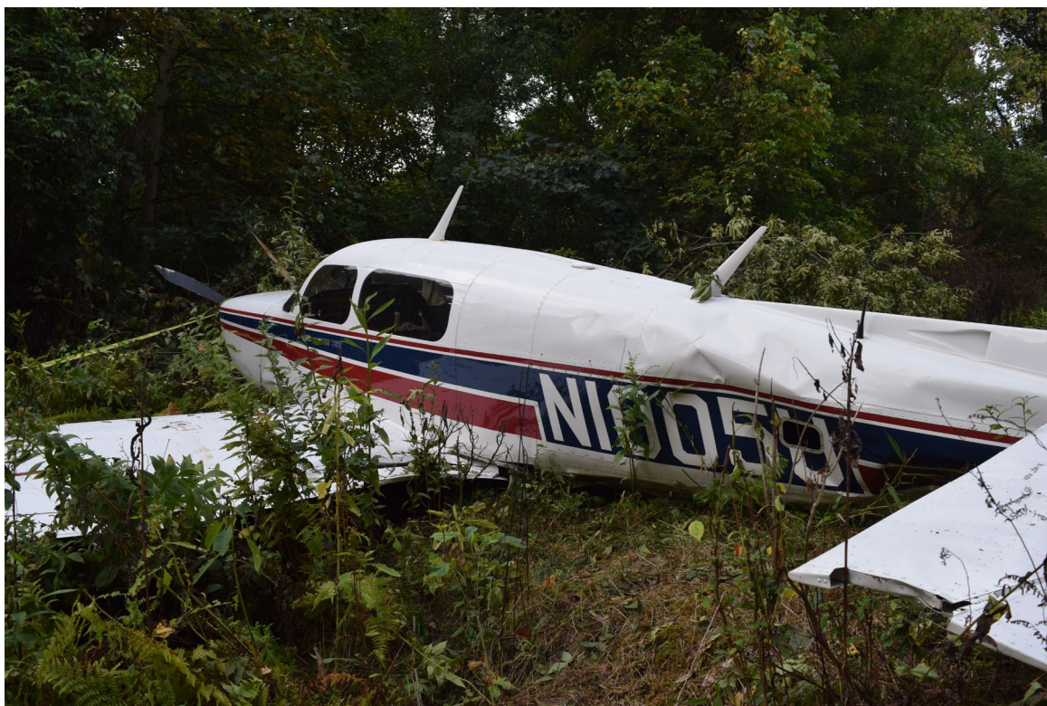
Photograph 2 - FAA Digital Photograph. Left Rear Quartering View of the Airplane At the Accident Site. Note the Compression Wrinkles in the Left Side of the Fuselage
