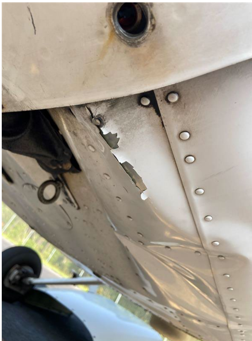
Photograph 2 - Fuselage buckling impact damage (Courtesy of FAA)
