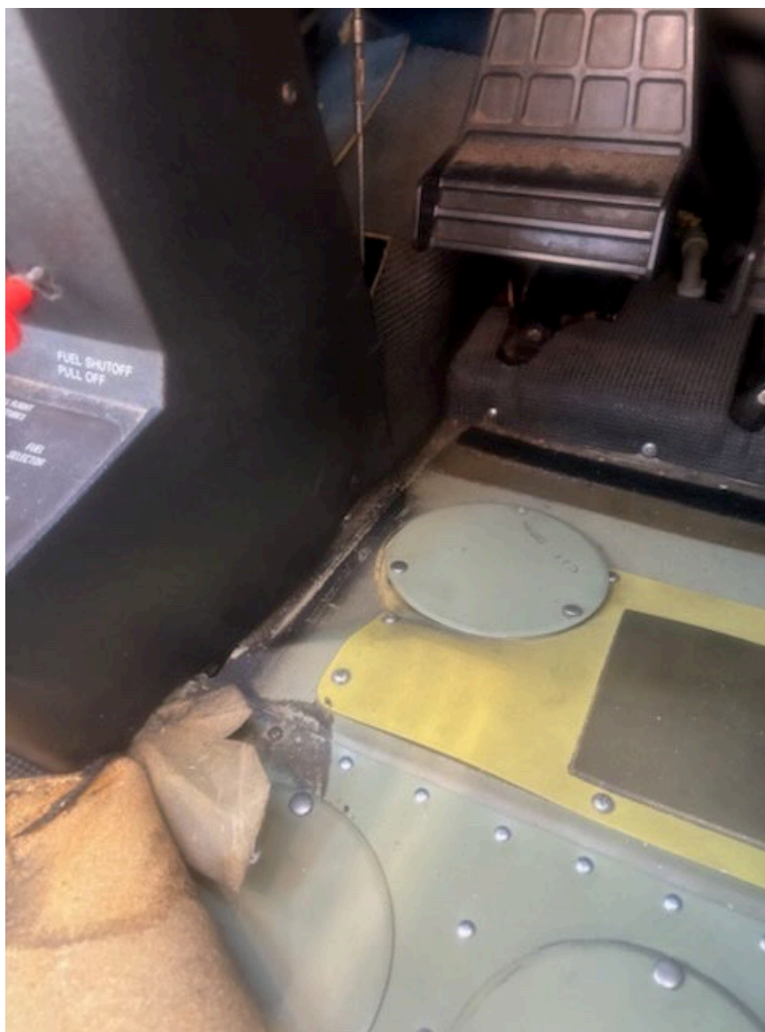
Photograph 4 - Floorboard buckling impact damage (Courtesy of FAA)
