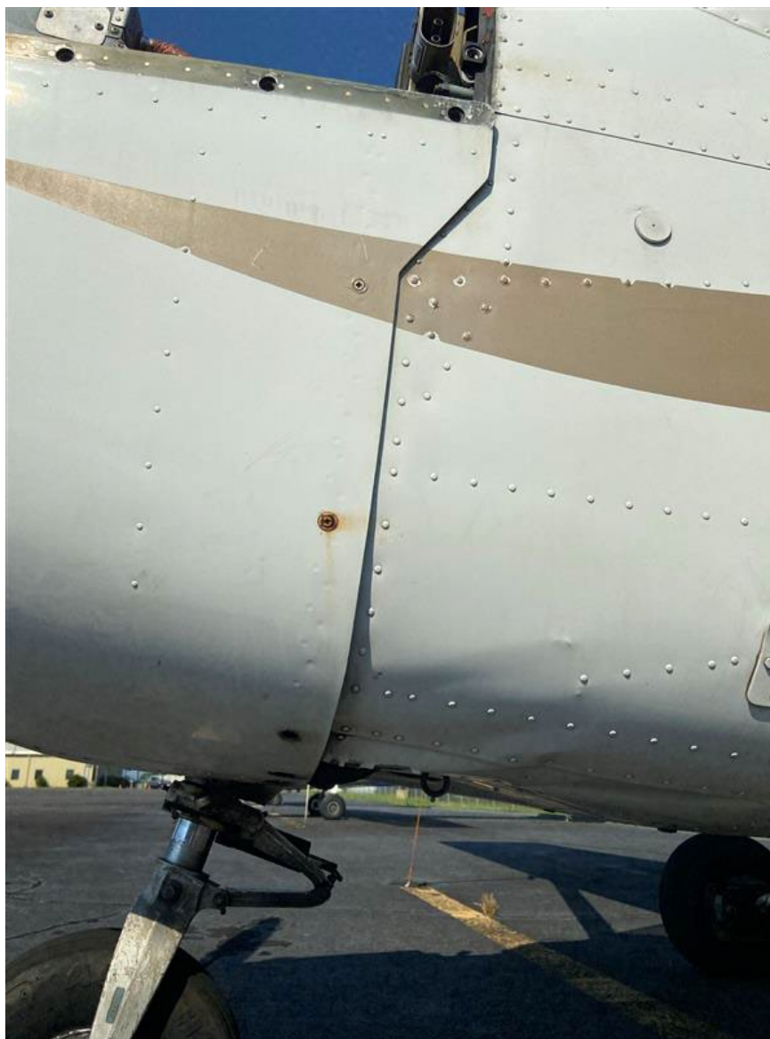
Photograph 1 - Fuselage buckling impact damage (Courtesy of FAA)
