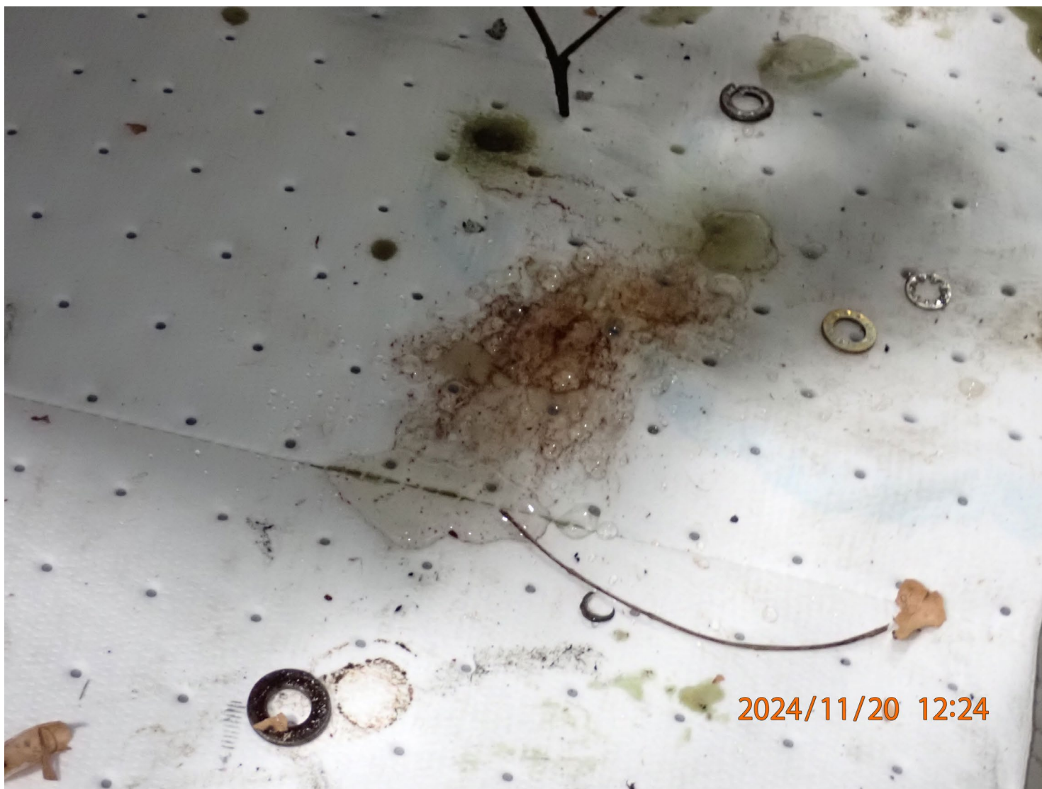
Photograph 3 - Evidence of Contaminated Fuel from Fuel Strainer
