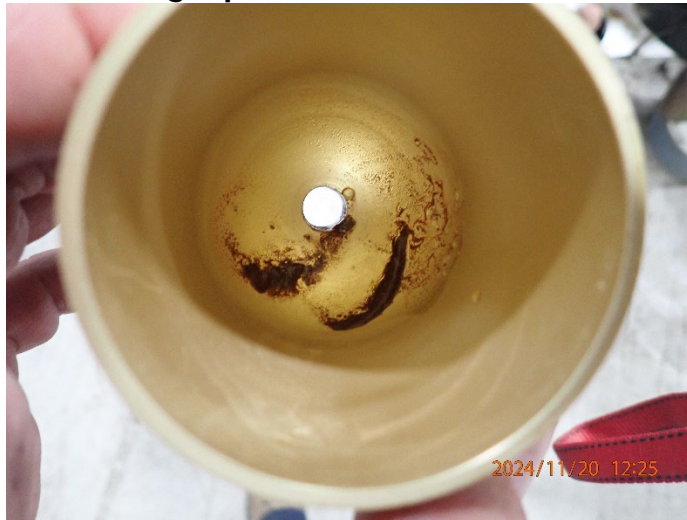
Fuel Strainer Bowl with Debris
