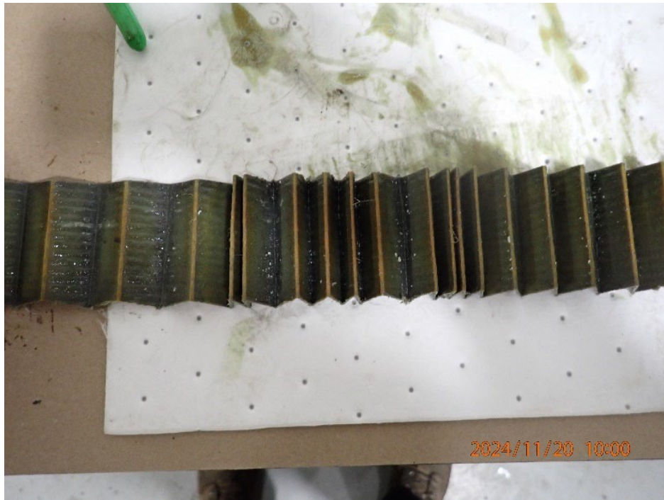
Oil Filter Element with Visible Assembly Lubrication
