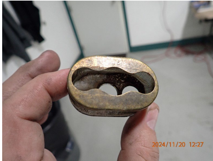
Debris in the Fuel Filter
