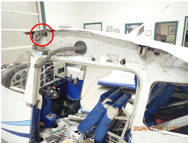
Plugged Left Wing Vent
