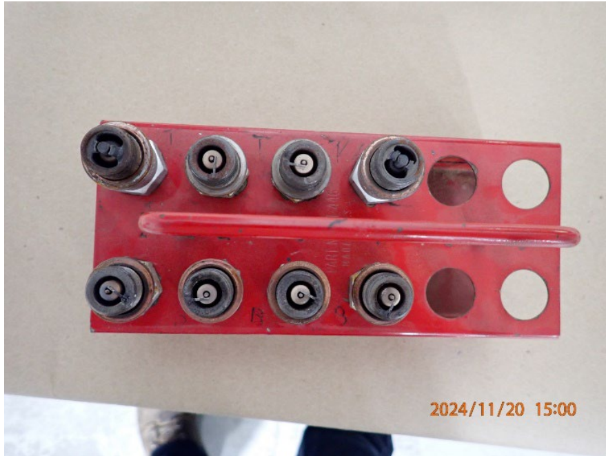
Spark Plugs as Removed
