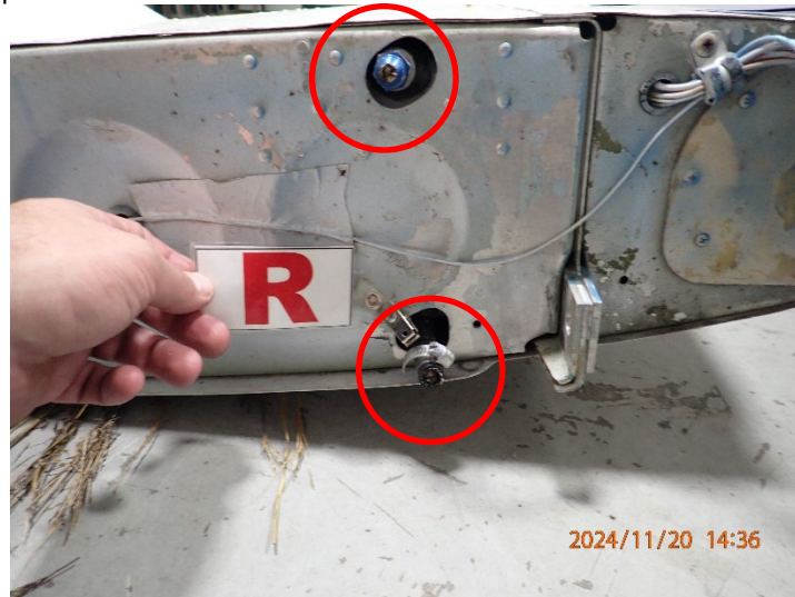
Plugged Fuel Lines from Recovery Personnel
