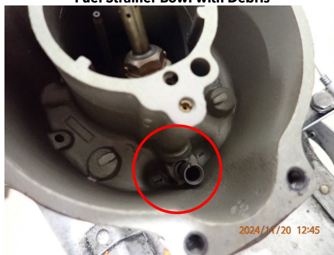
Debris in the Carburetor Bowl
