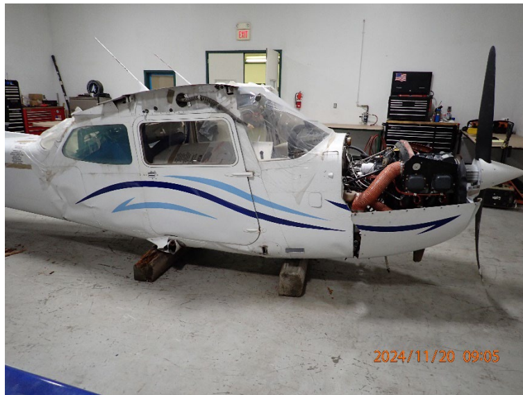
Right Side Fuselage Wrinkling
