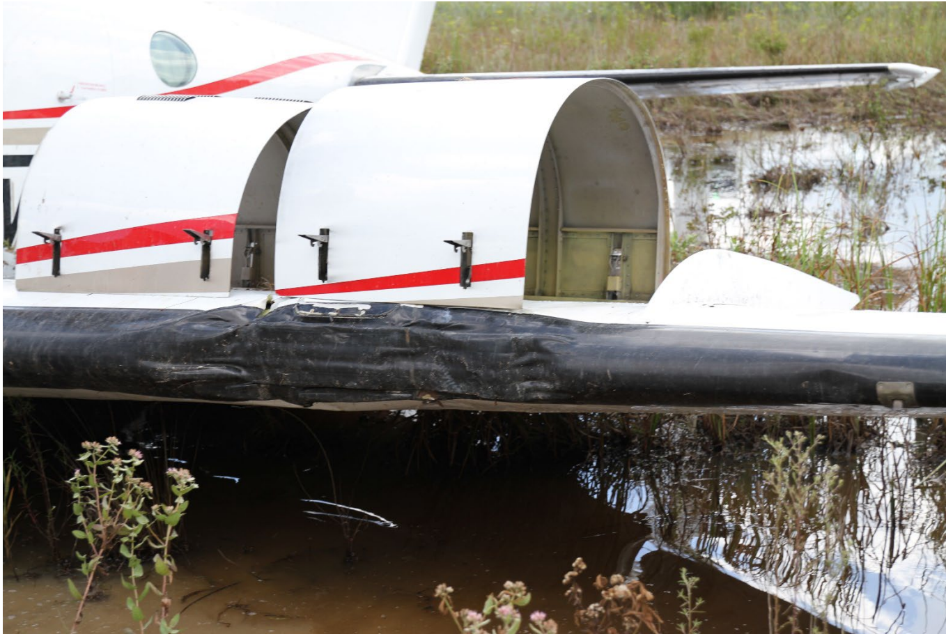
Photograph 2 - View of Airplane's Left Wing Damage (Courtesy of FAA)
