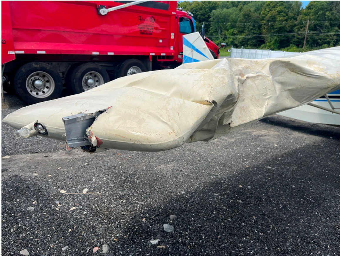
Photograph 2 - Damage to right wing (Courtesy of FAA)
