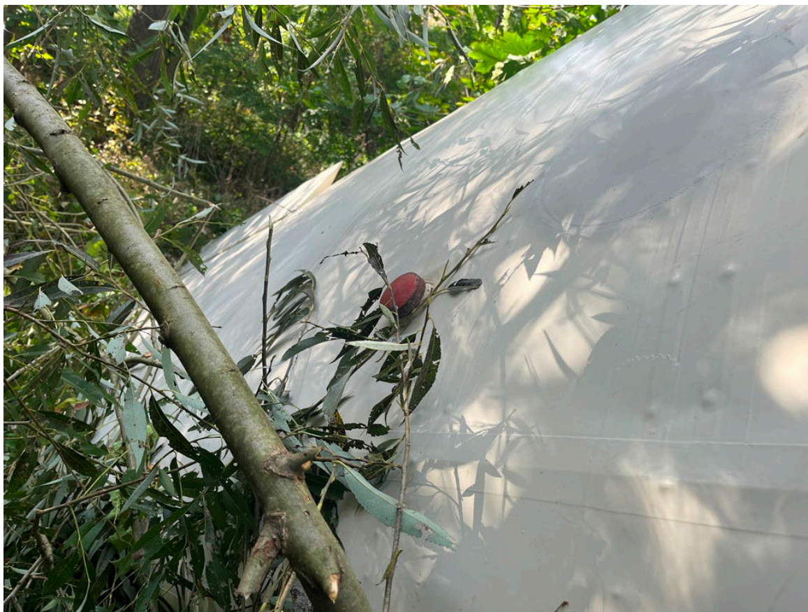
Photograph 5 - Top of right wing - Fuel cap intact (Courtesy of FAA)
