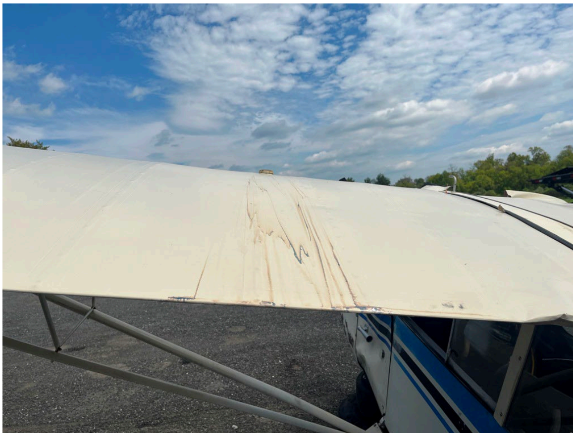
Photograph 4 - Fuel streaking aft of fuel cap - Left wing (Courtesy of FAA)
