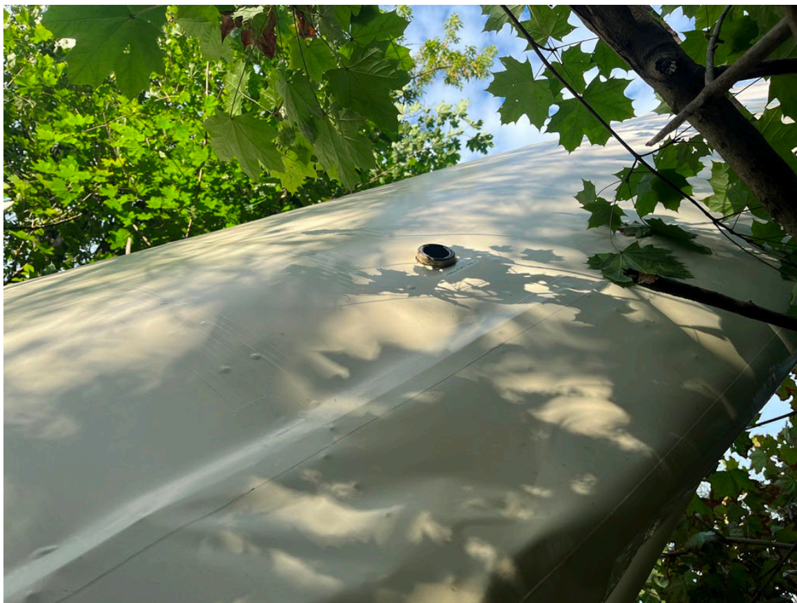
Photograph 3 - Top of left wing - Fuel cap missing (Courtesy of FAA)
