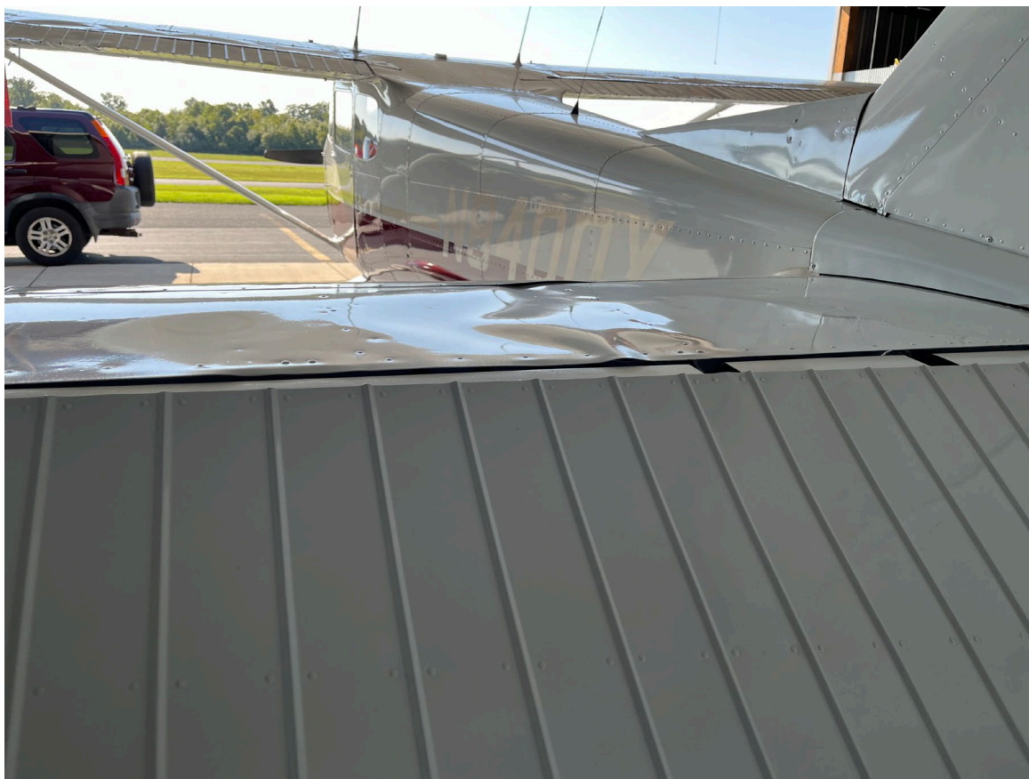
Photograph 1 - Accident horizontal stabilizer damage (Courtesy of FAA)
