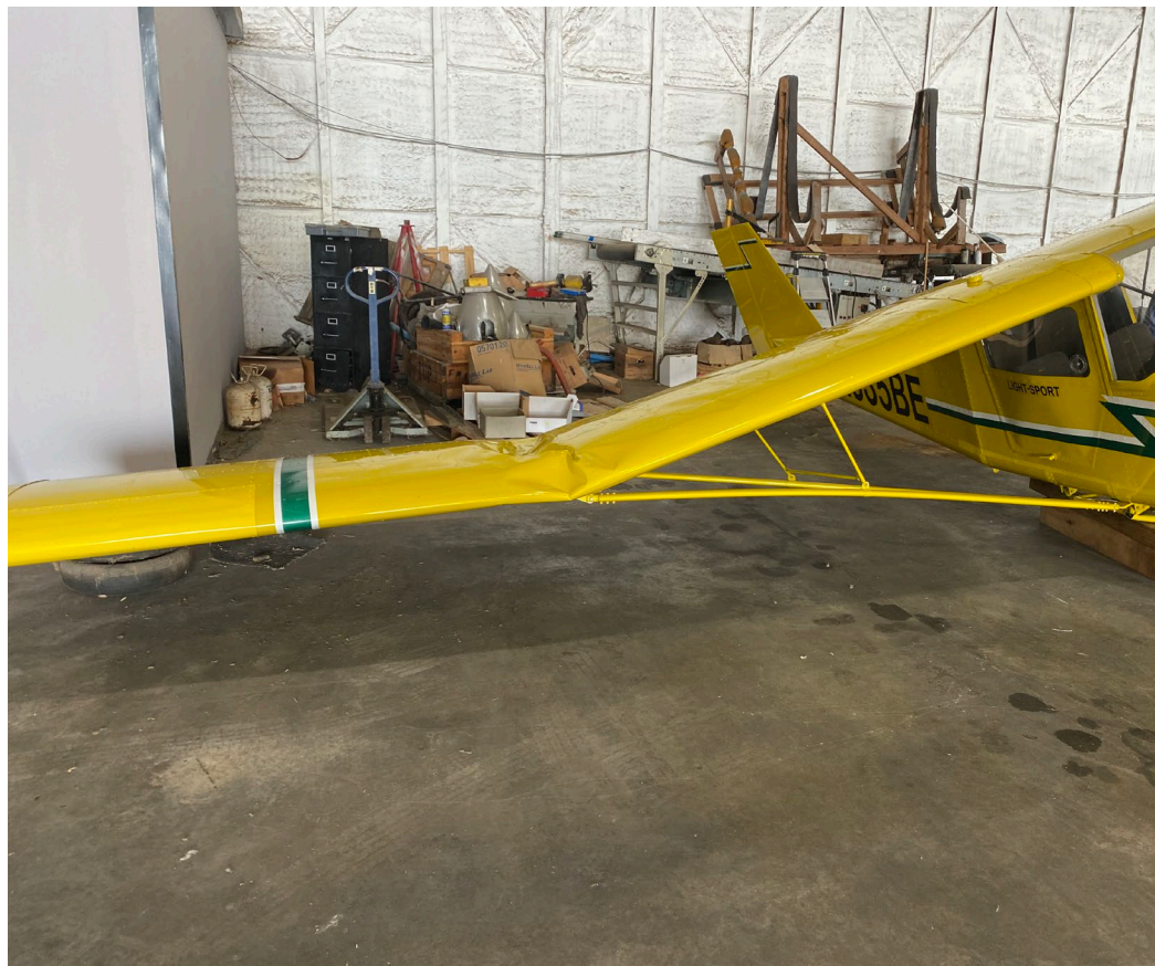
Photograph 3 - Right wing impact damage (Courtesy of FAA)
