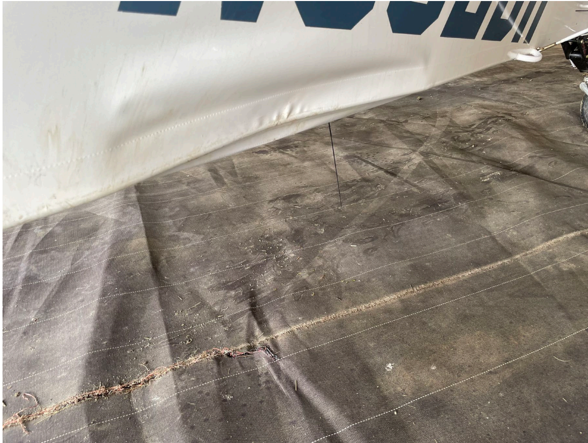
Photograph 2 - View of damage to the left side of the fuselage. (Courtesy of FAA)
