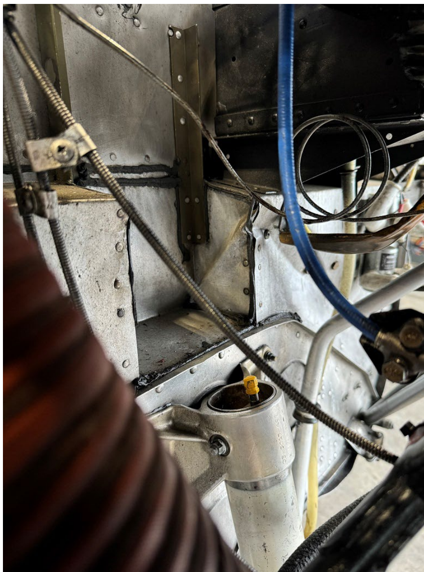
Photograph 2 - Tunnel Structure Substantial Damage (Courtesy of FAA)
