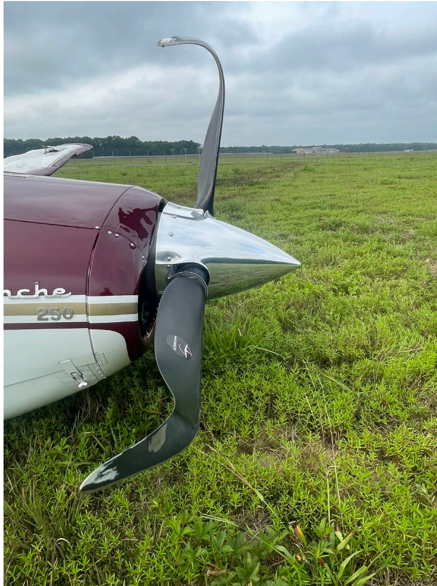
Photograph 3 - Propeller Damage (Courtesy of FAA)
