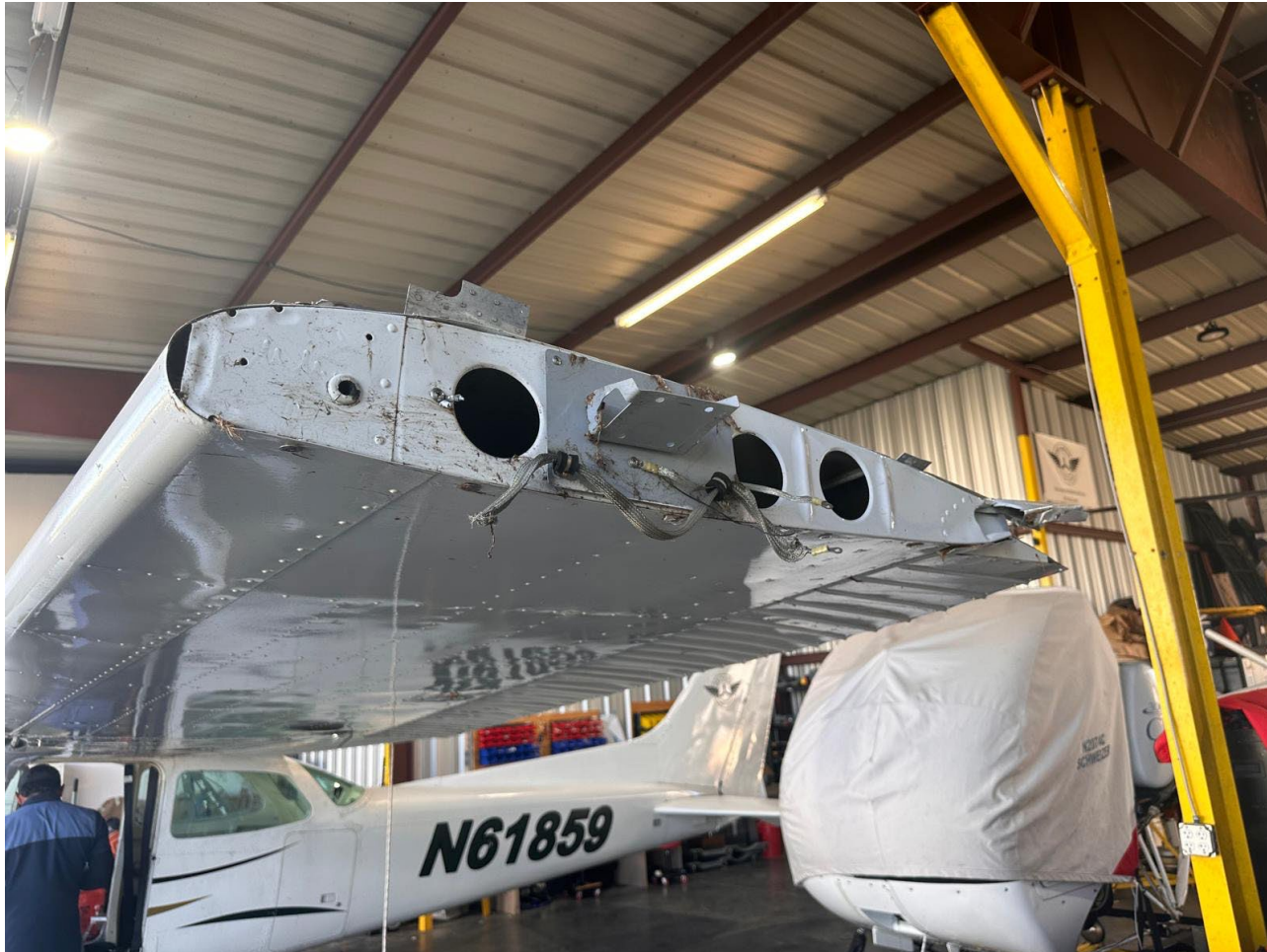
Photograph 3 - Left wingtip damage. (Courtesy of FAA)
