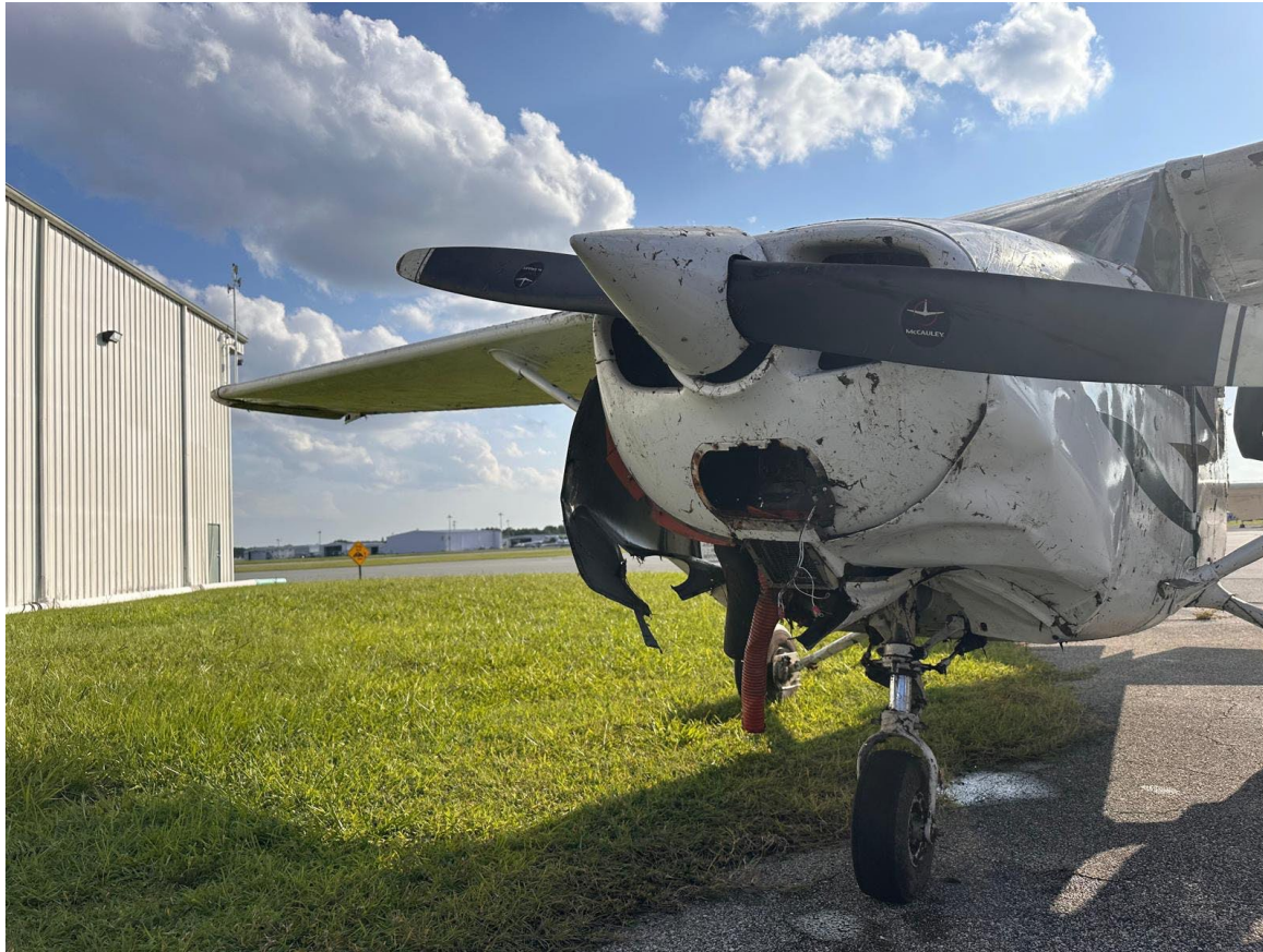
Photograph 2 - Fuselage and engine compartment damage. (Courtesy of FAA)
