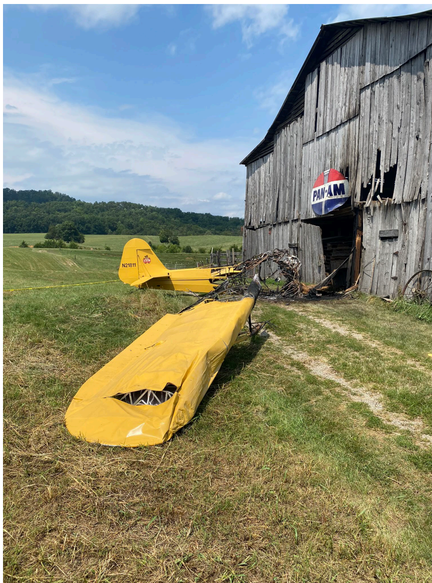
Photograph 1 - Deformation noted to fuselage tubular structure (Courtesy of FAA)
