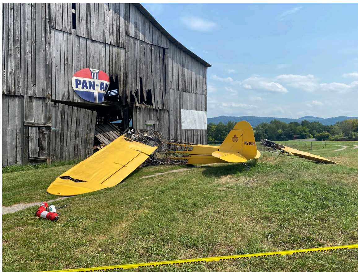
Photograph 2 - Tubular structure deformation and thermal damage noted (Courtesy of FAA)
