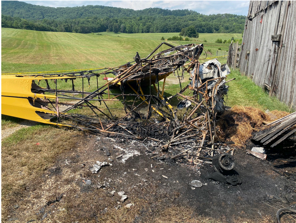
Photograph 3 - Thermal damage noted to fuselage (Courtesy of FAA)
