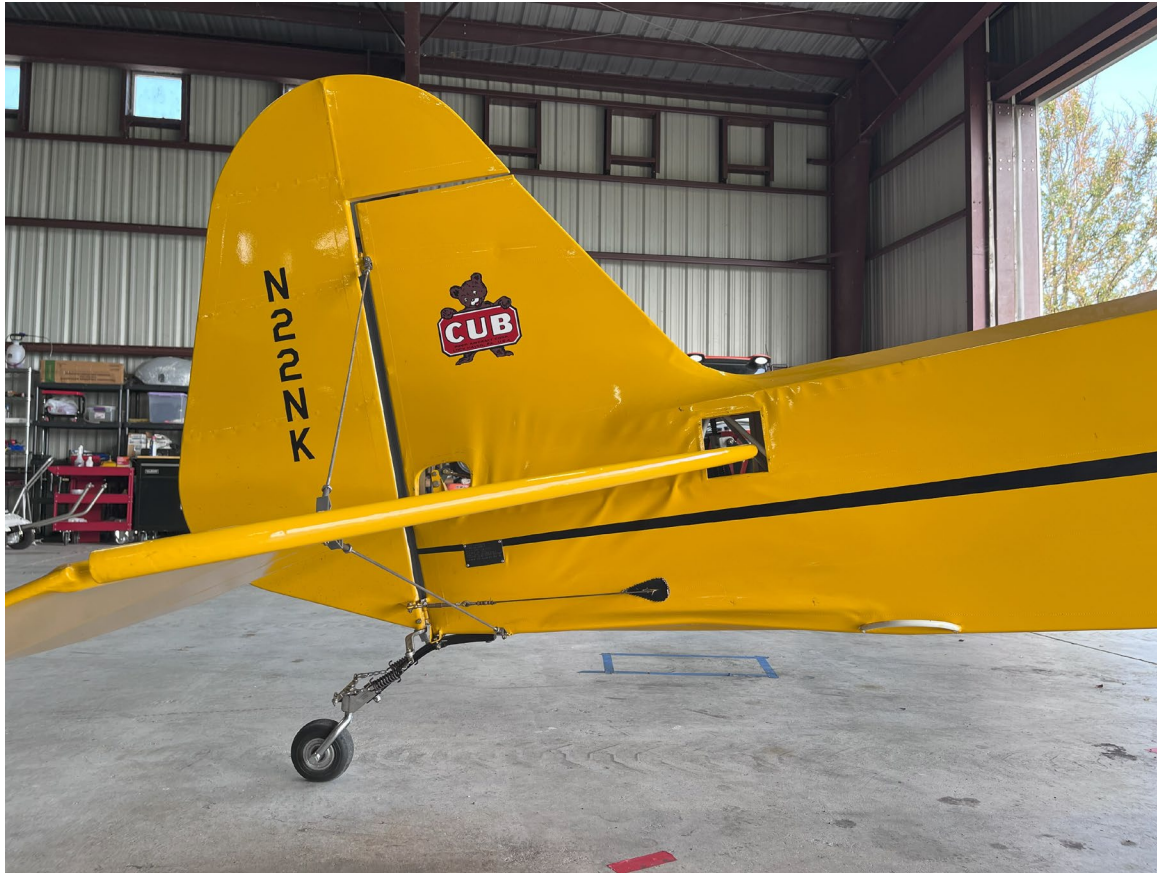
Photograph 4 - Digital Photograph From Owner. Right Side View of the Aft Empennage. Note the Wrinkle in the Fabric on the Lower Fuselage Tubing
