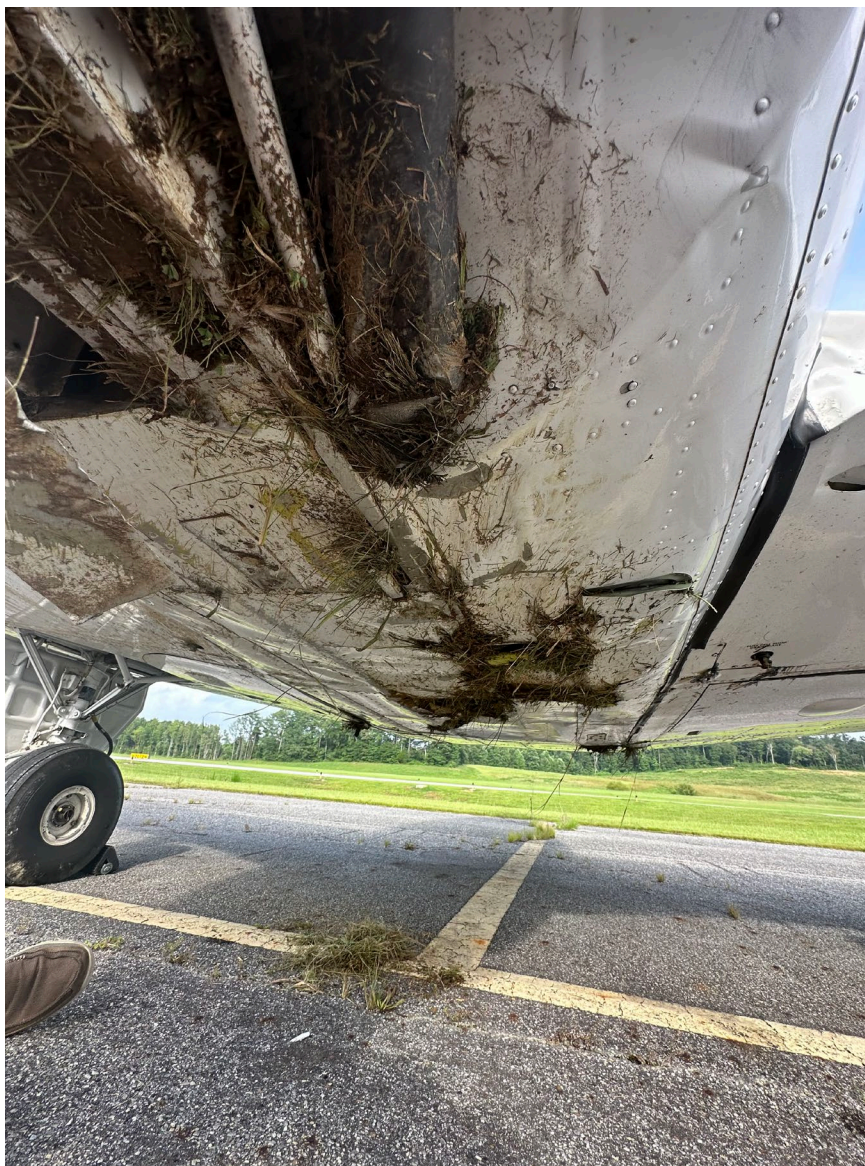
Photograph 2 - Deformation noted to the fuselage skin (Courtesy of FAA)
