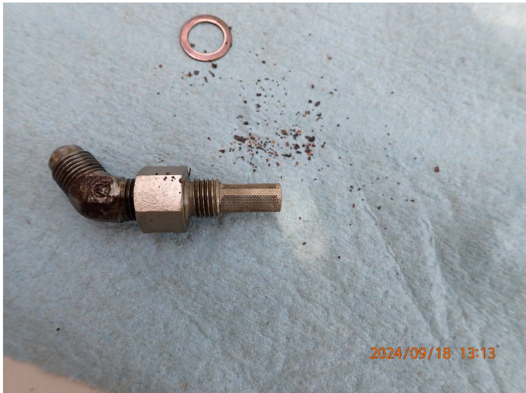
Photo 3: View of the carburetor fuel inlet screen with debris from in the screen.
