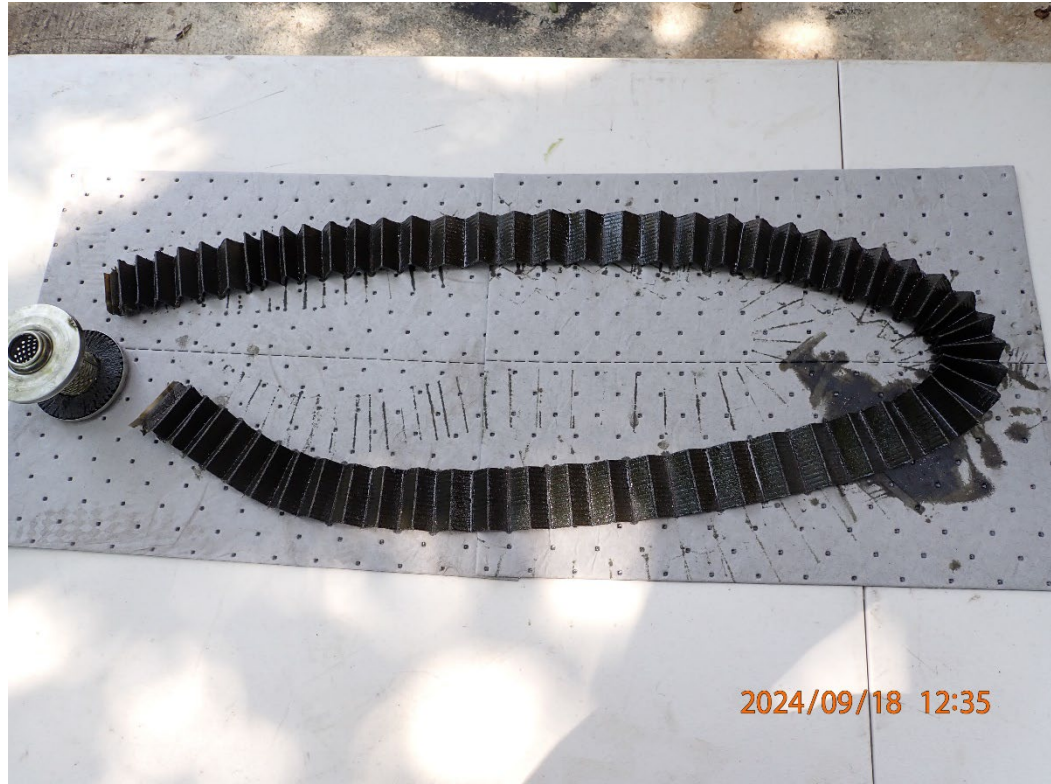
Photo 5: View of the oil filter cut open for examination.
