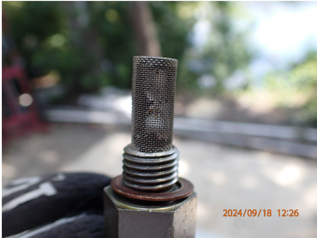
Photo 2: View of the carburetor fuel inlet screen.
