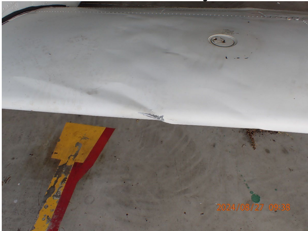
Photo 13: View of damage to the left wing.
