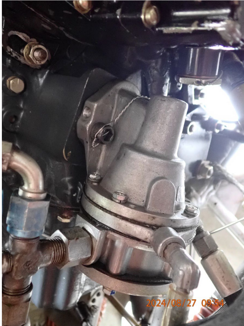
Photo 36: View of the engine driven fuel pump secure in the accessory case.
