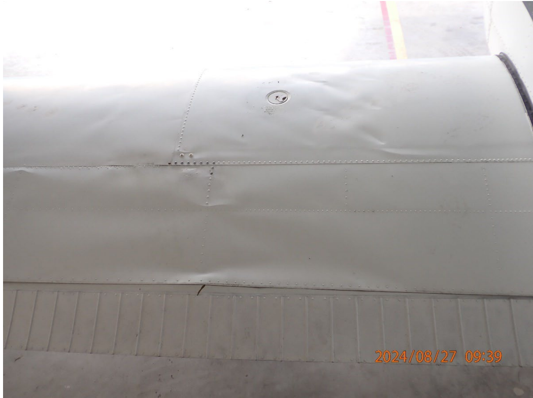
Photo 14: View of damage to the left wing.
