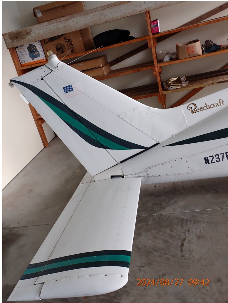
Photo 7: View of the right stabilator with trim tab, rudder, and vertical stabilizer.
