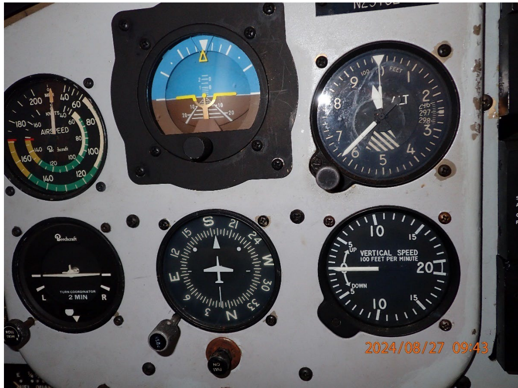
Photo 20: View of the six primary flight instruments.
