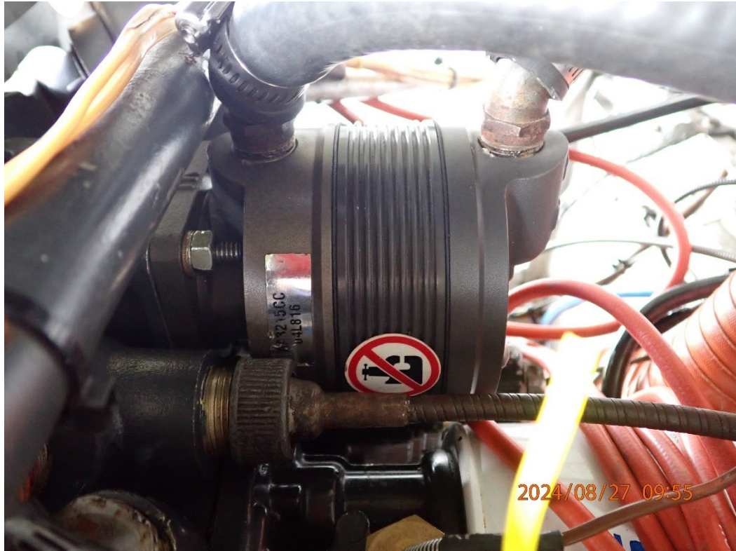
Photo 39: View of the vacuum pump secure in the accessory case.
