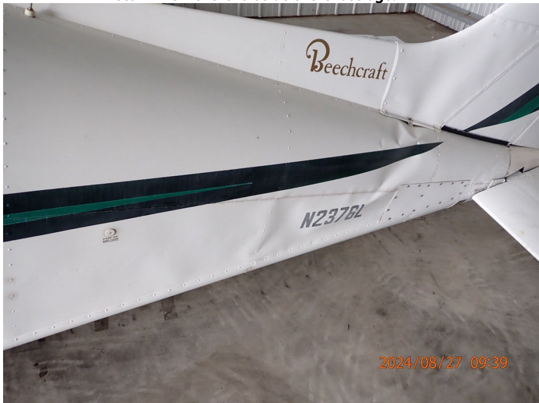
Photo 2: View of damage to the left side of the fuselage.
