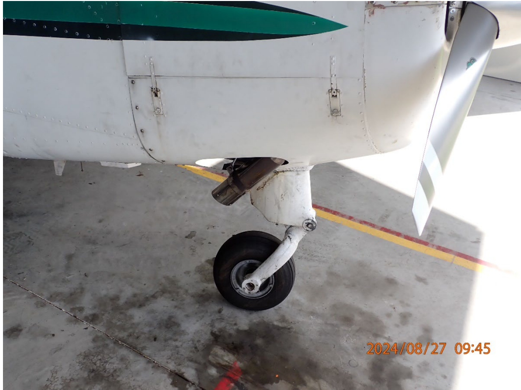
Photo 32: View of the undamaged exhaust.
