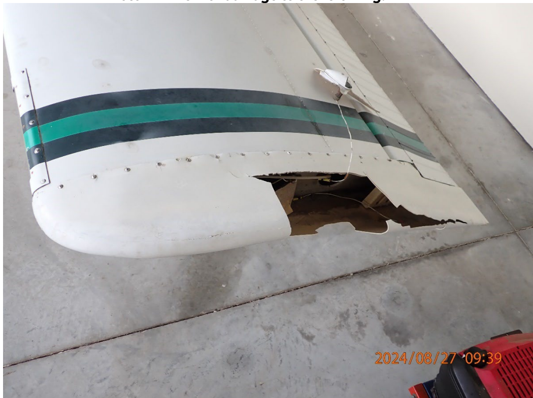
Photo 15: View of damage to the left wing tip.
