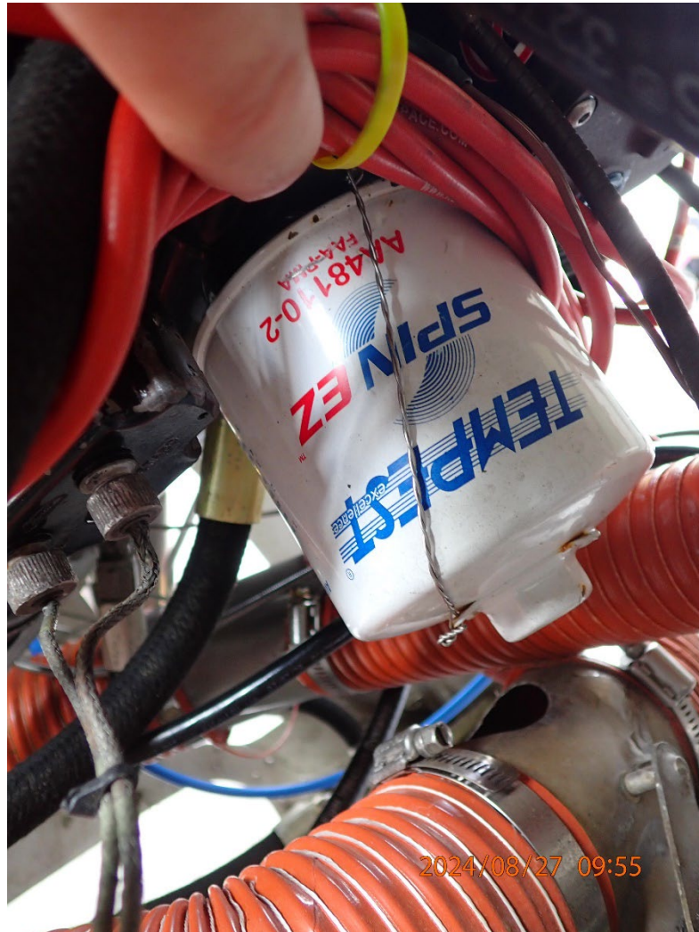
Photo 37: View of the oil filter secure with safety wire on its mount.
