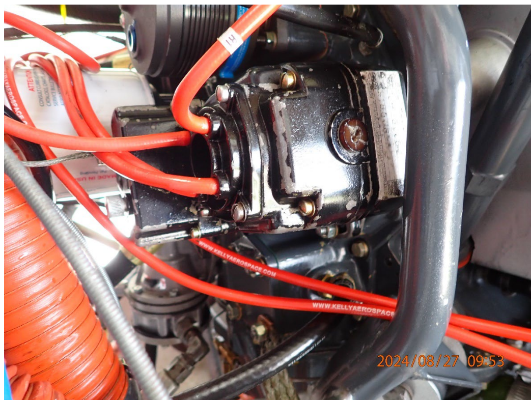
Photo 33: View of the right magneto secure in the accessory case.
