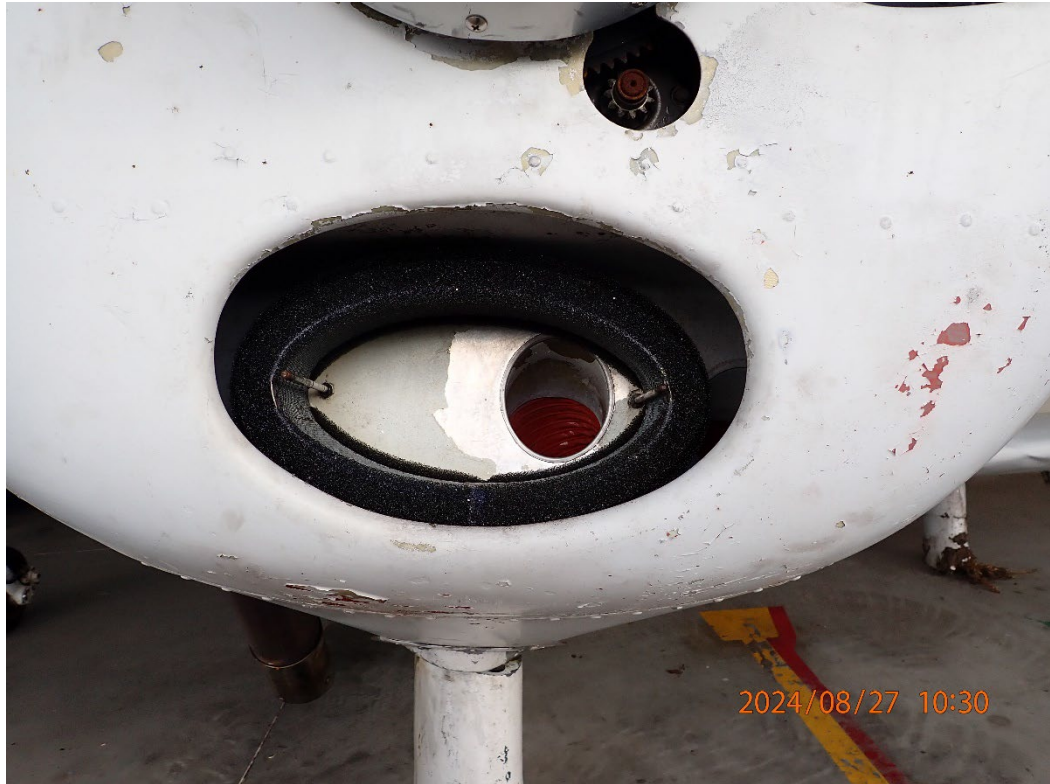
Photo 30: View of the air intake filter in place in the nose.
