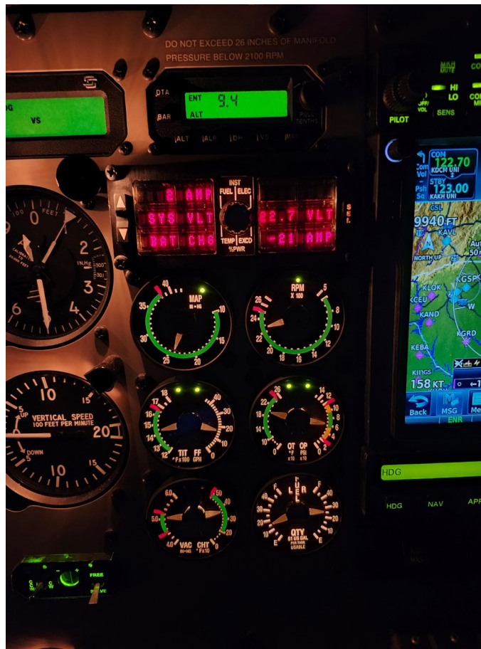
Photograph 5 - Electrical power depiction after alternator failure and before battery failure in flight (Courtesy of Pilot)
