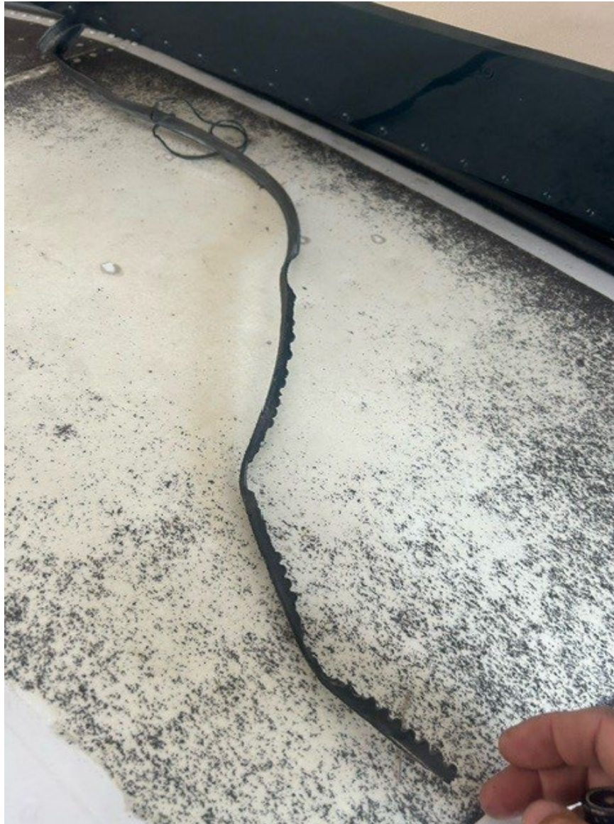
Photograph 4 - Shredded alternator belt (Courtesy of FAA)
