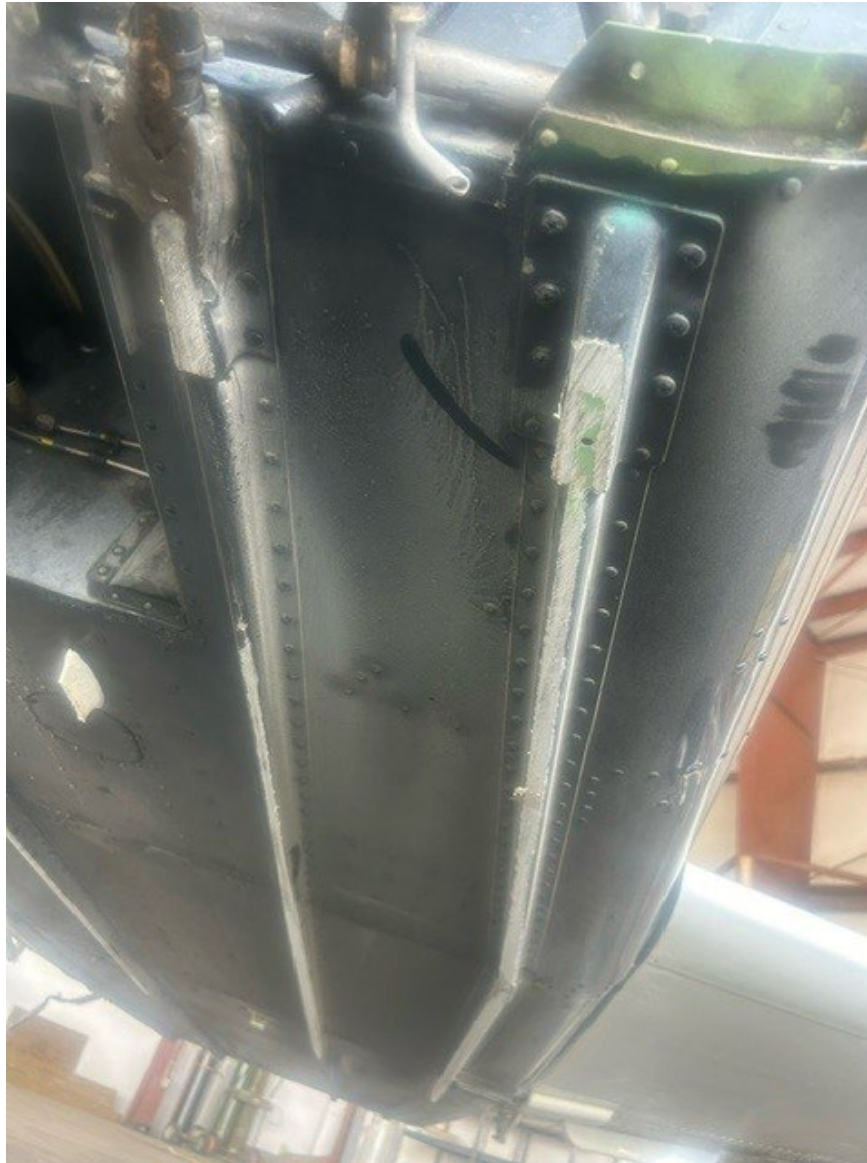
Photograph 2 - Damage to external longerons (Courtesy of FAA)
