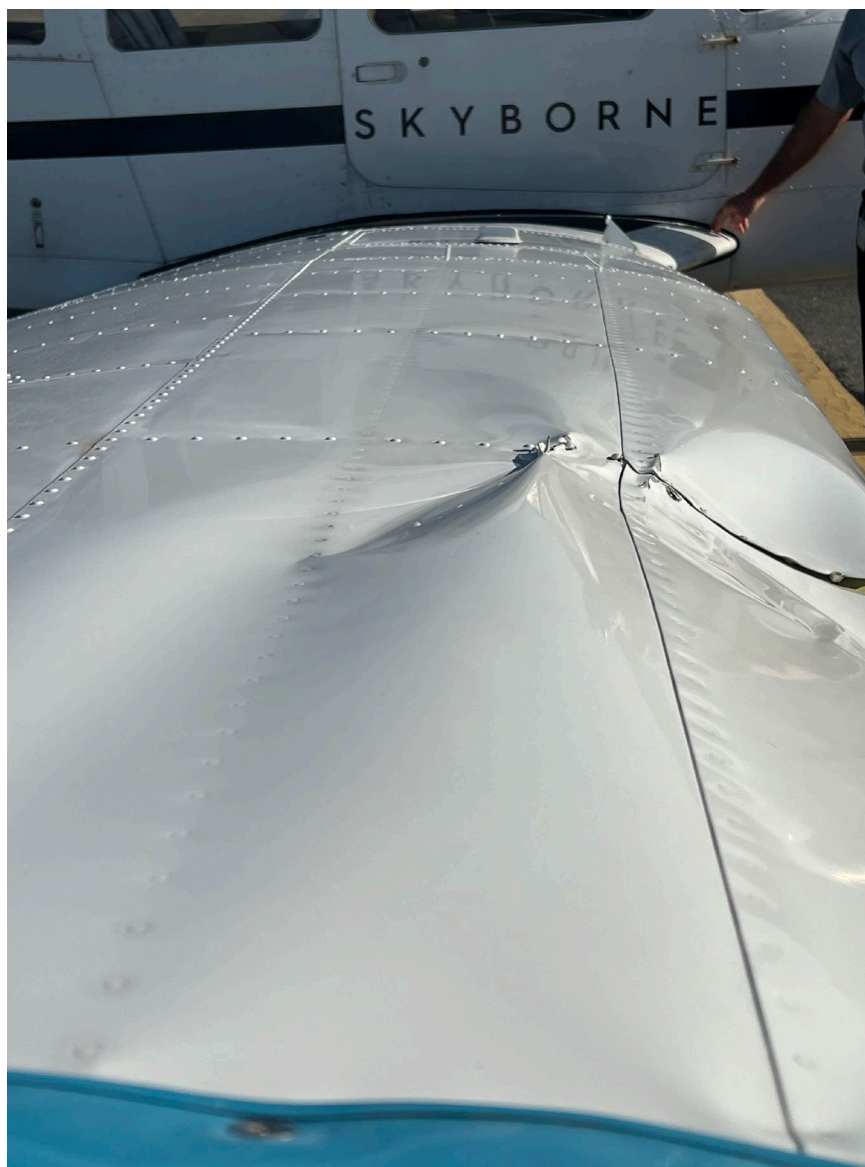
Photograph 4 - Damage to low-wing airplane's wing (Courtesy of Skyborne Airlines)
