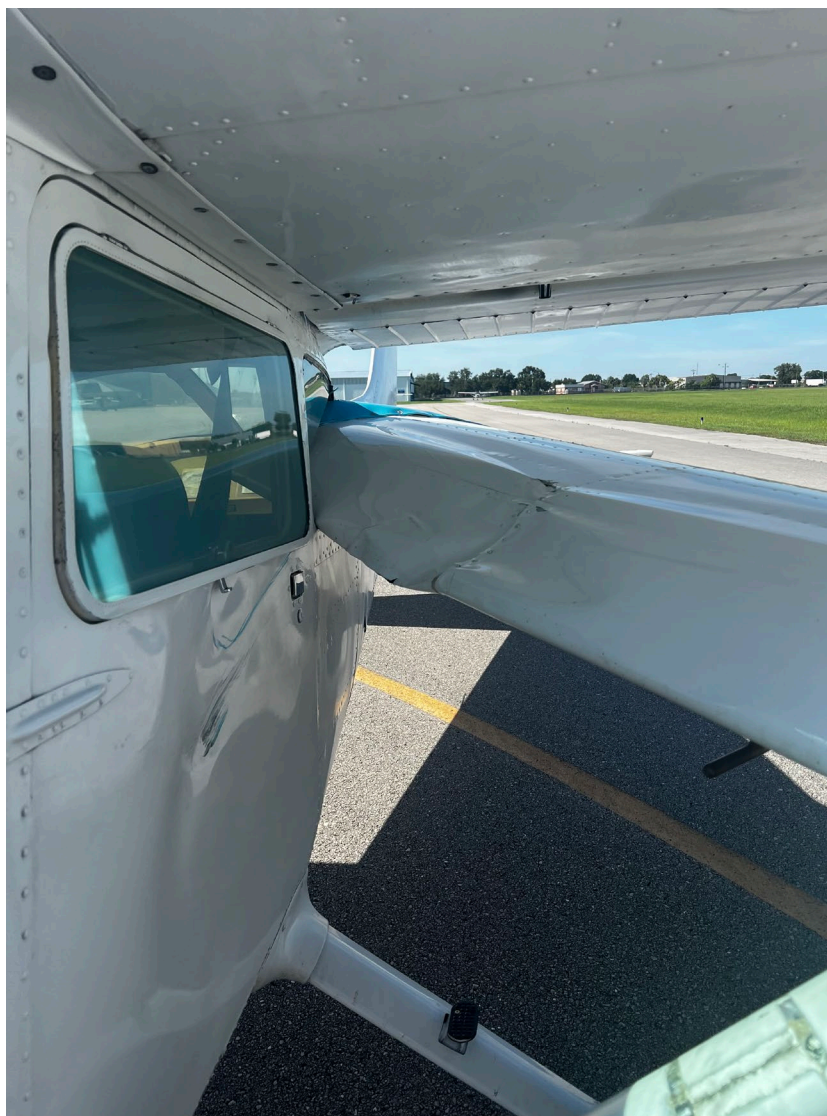
Photograph 3 - Postaccident view of low-wing's wing broken through high-wing's window (Courtesy of Skyborne Airlines)
