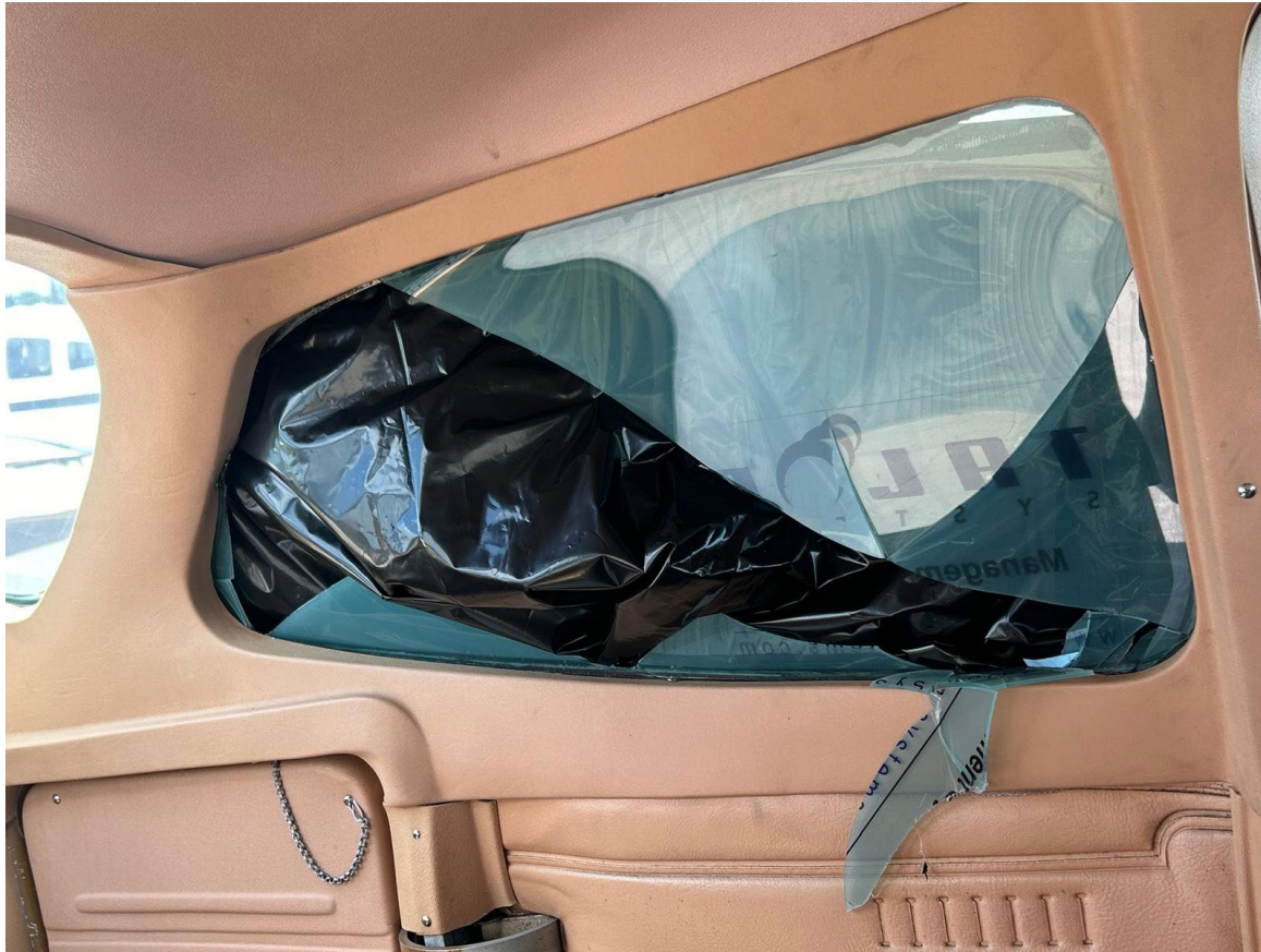
Photograph 7 - Damage to high wing airplane's window (Courtesy of Wayman Aviation)
