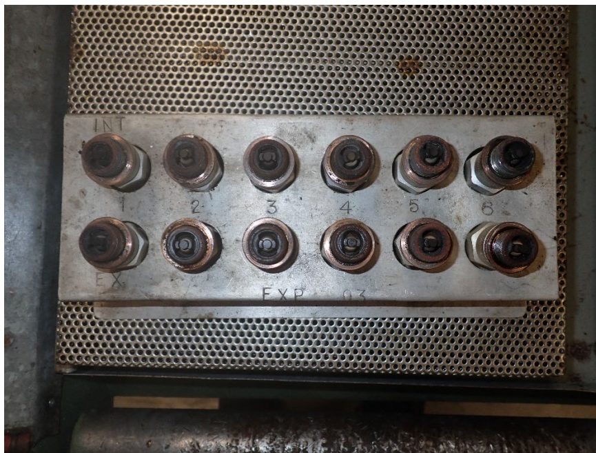
Photograph 3 - Spark plugs showing carbon fouling on cylinder No. 6. (Courtesy of Lycoming)
