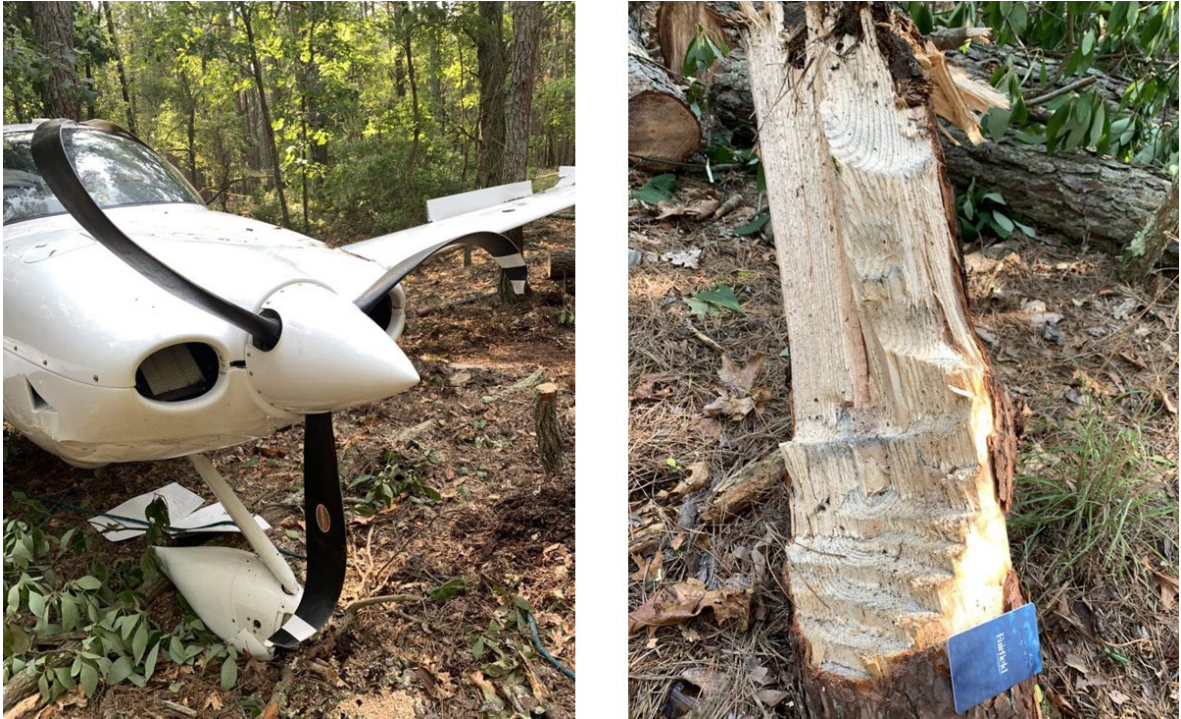
Figure 1 Accident site, damage and tree propeller chopping/cutting marks.
