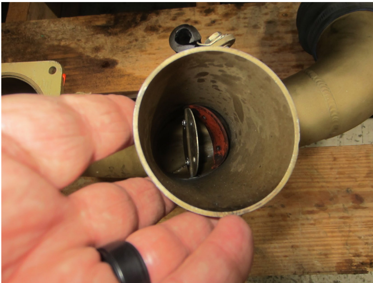
Photograph 6 - Half of the alternate air valve partially installed in induction tube. (NTSB)
