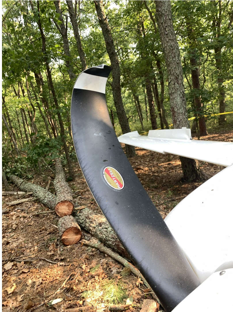
Photograph 2 - Closeup view of propeller damage. (Courtesy of FAA)
