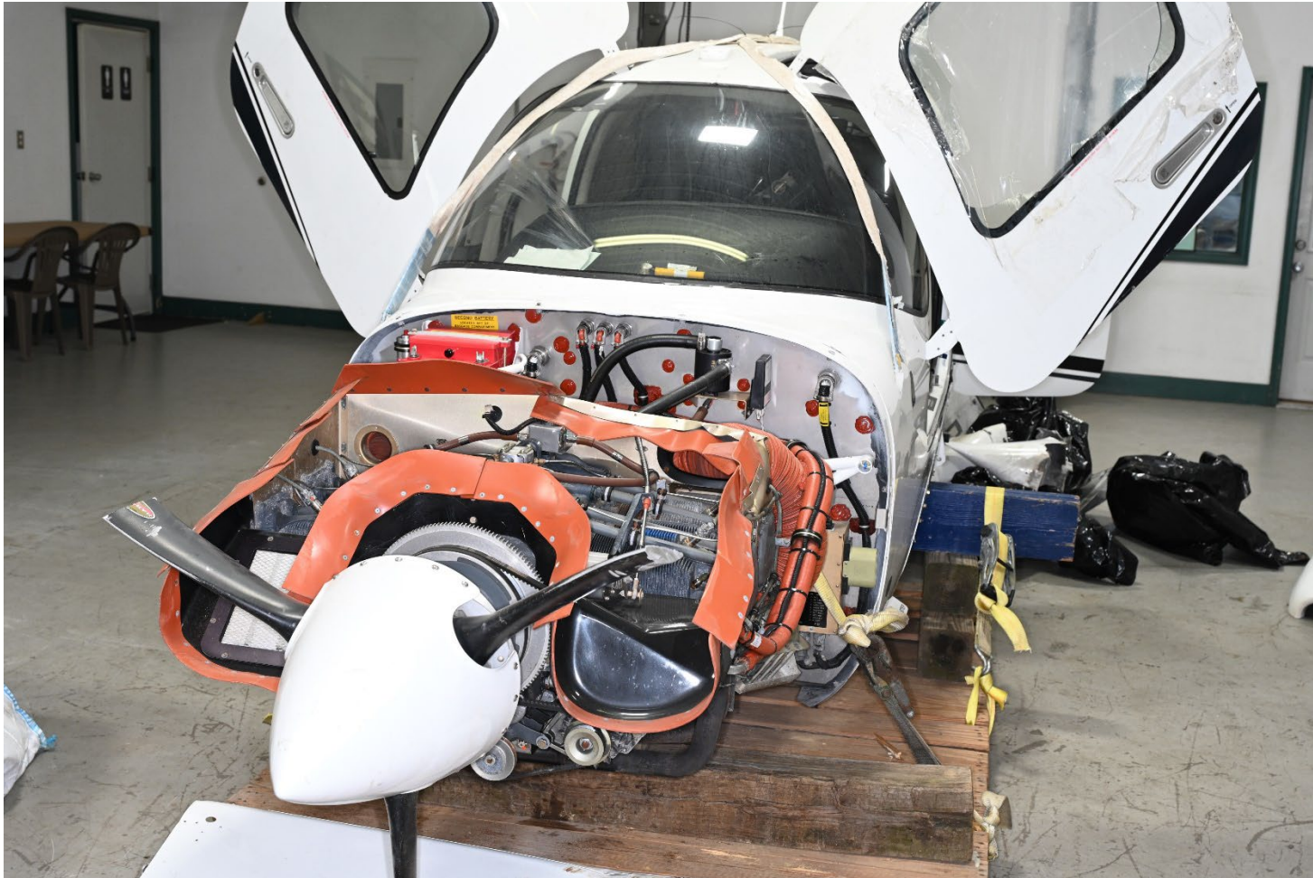
Photograph 4 - Airplane prior to full examination. Note propellers cut off equally to facilitate safe engine run. (NTSB)
