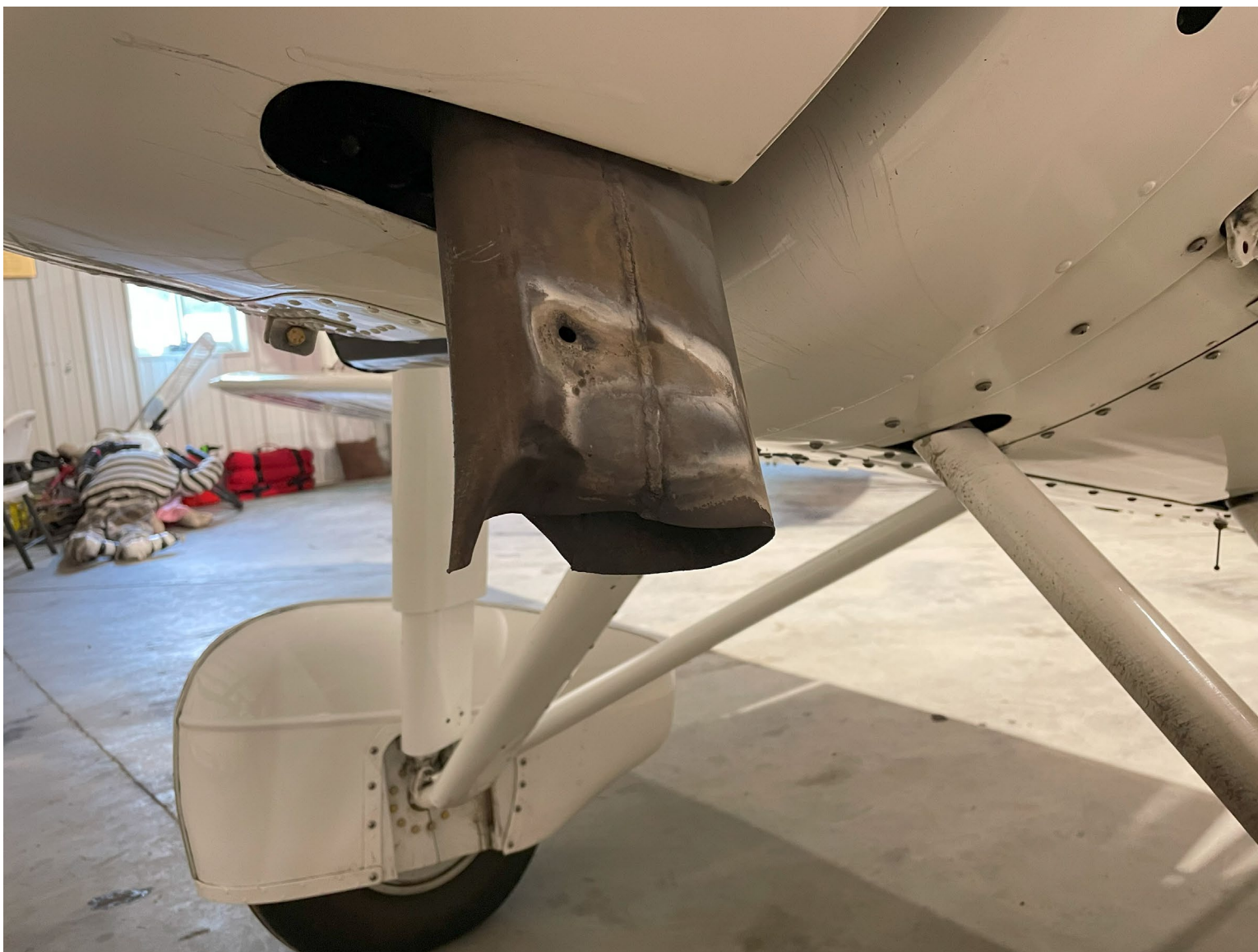
Photograph 6 – Damage to exhaust pipe of N108CH (Courtesy of FAA)
