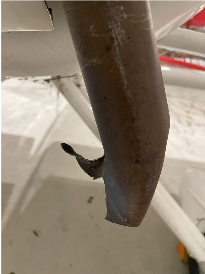
Photograph 7 - Damage to exhaust pipe of N108CH (Courtesy of FAA)
