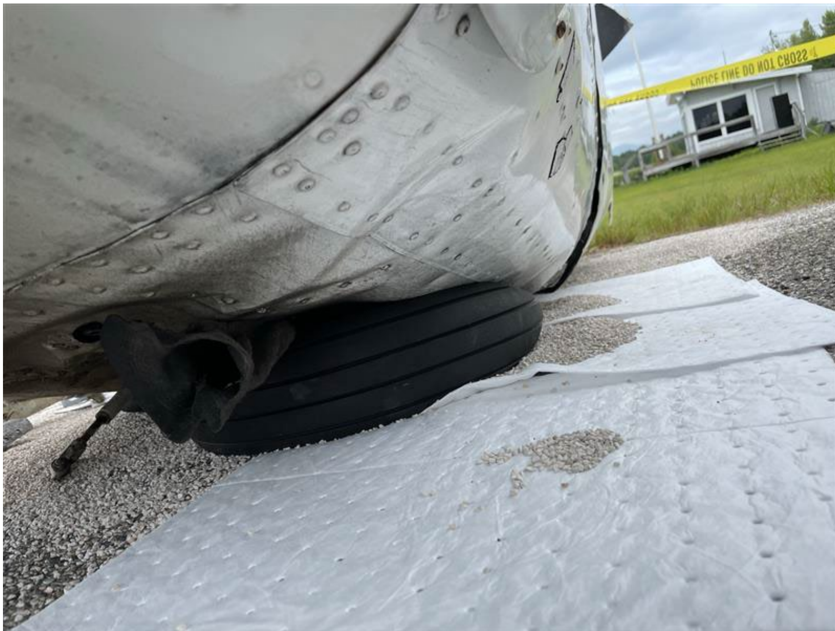
Photo 3 – View of Wrinkled Cabin Structure (FAA)
