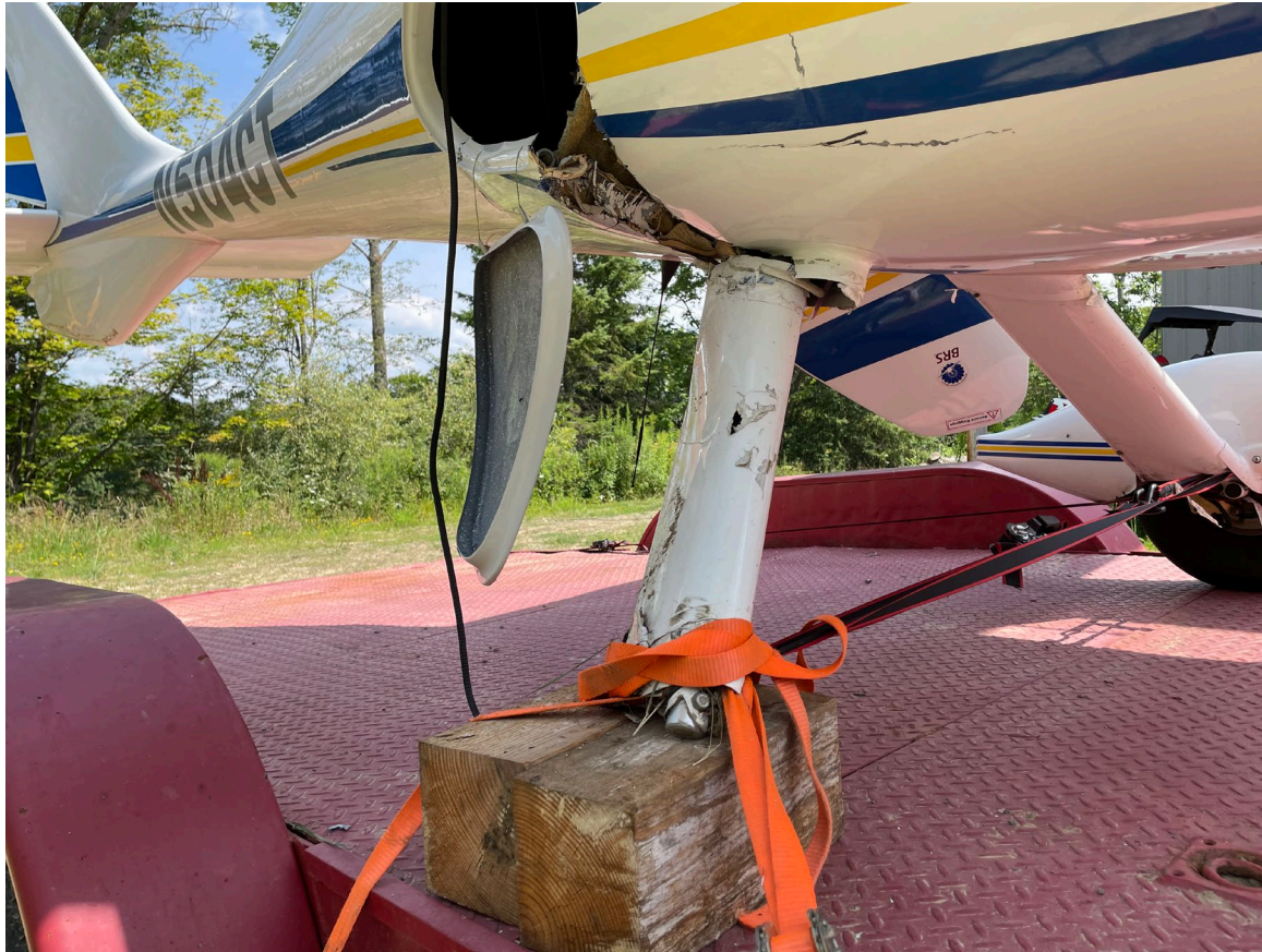
Photograph 1 - Postaccident damage right side lower fuselage (Courtesy of FAA)
