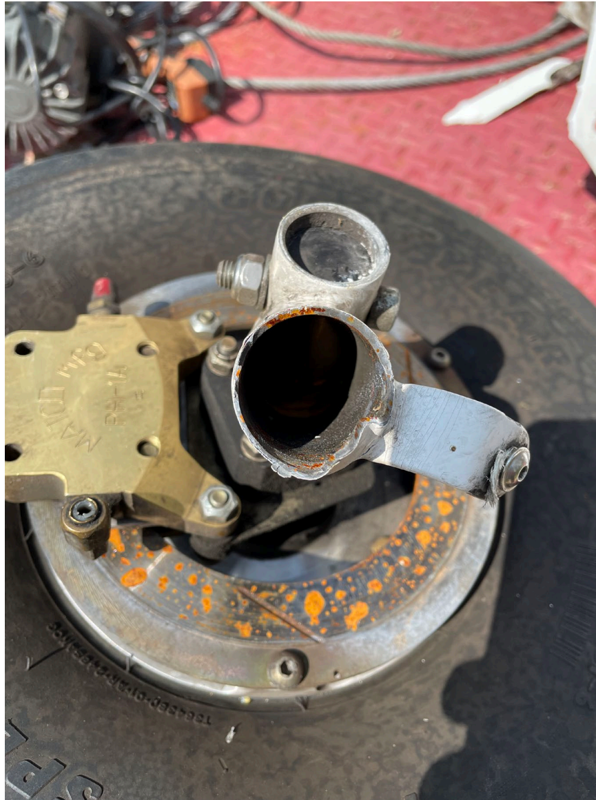
Photograph 2 - Postaccident damaged main wheel attach fitting (Courtesy of FAA)
