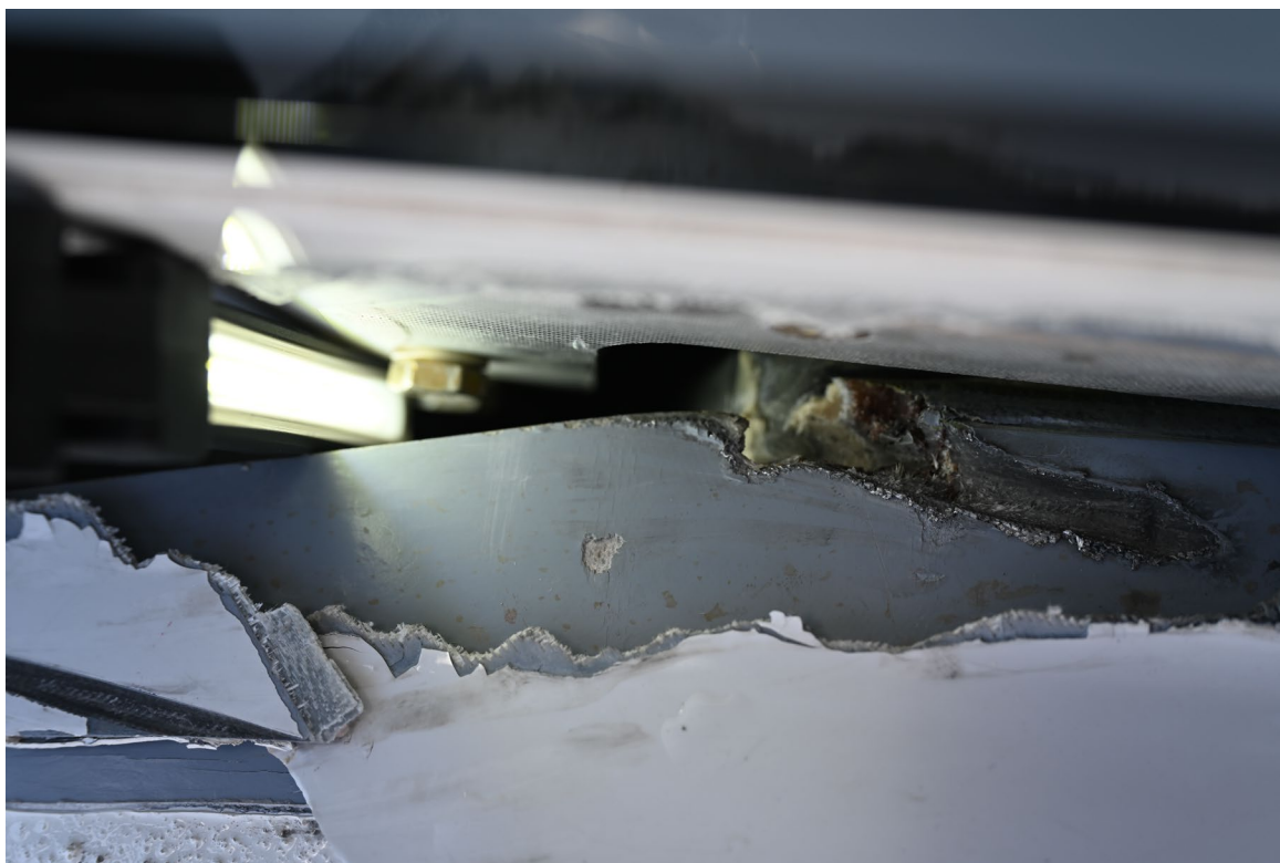
Photograph 2 - Left Wing Spar Damage (Courtesy of FAA)
