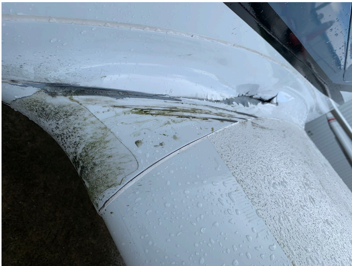
Photograph 1 - Left Wing Root External Damage (Courtesy of FAA)
