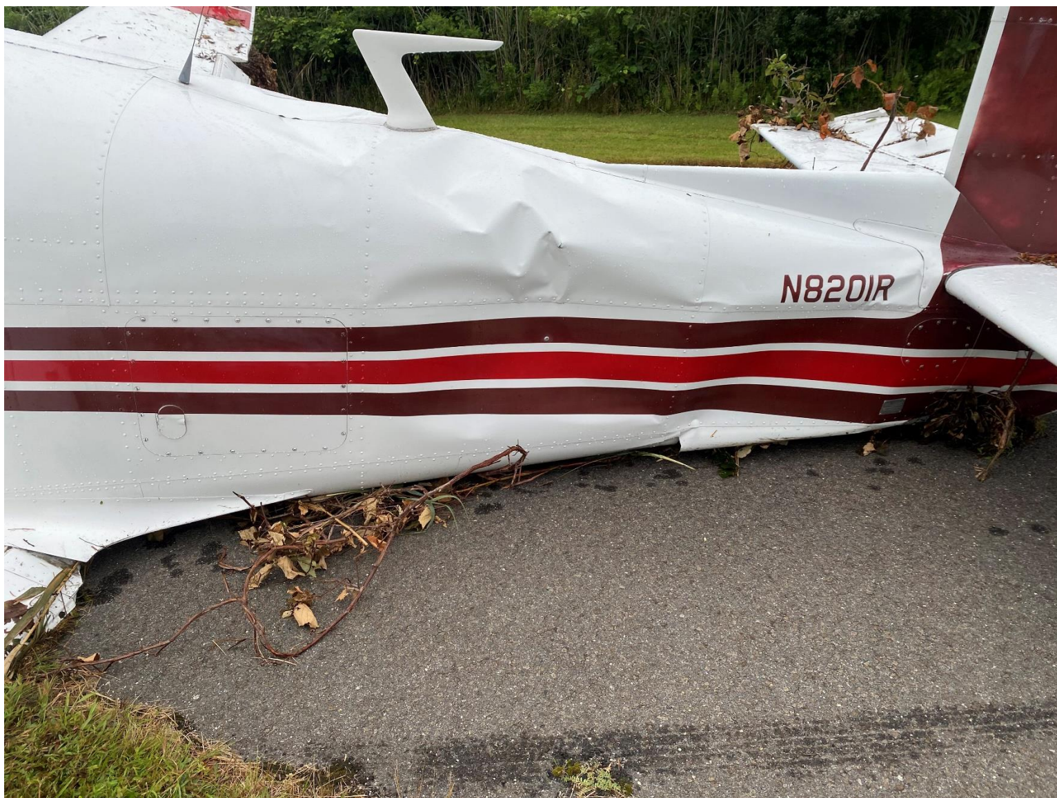
Photograph 3 – Damage to the fuselage (Courtesy of the pilot)
