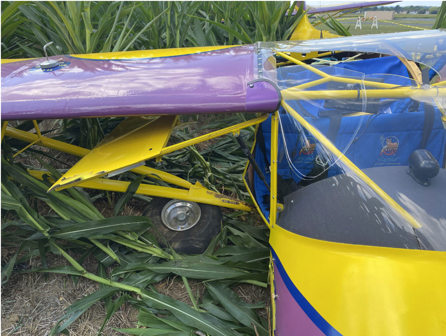
Photograph 5 - Damaged main landing gear (Courtesy of FAA)
