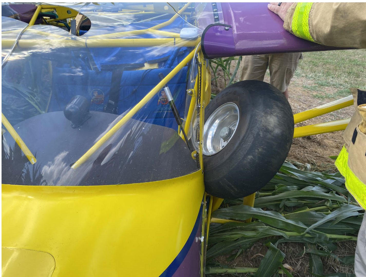
Photograph 4 - Damaged main landing gear (Courtesy of FAA)
