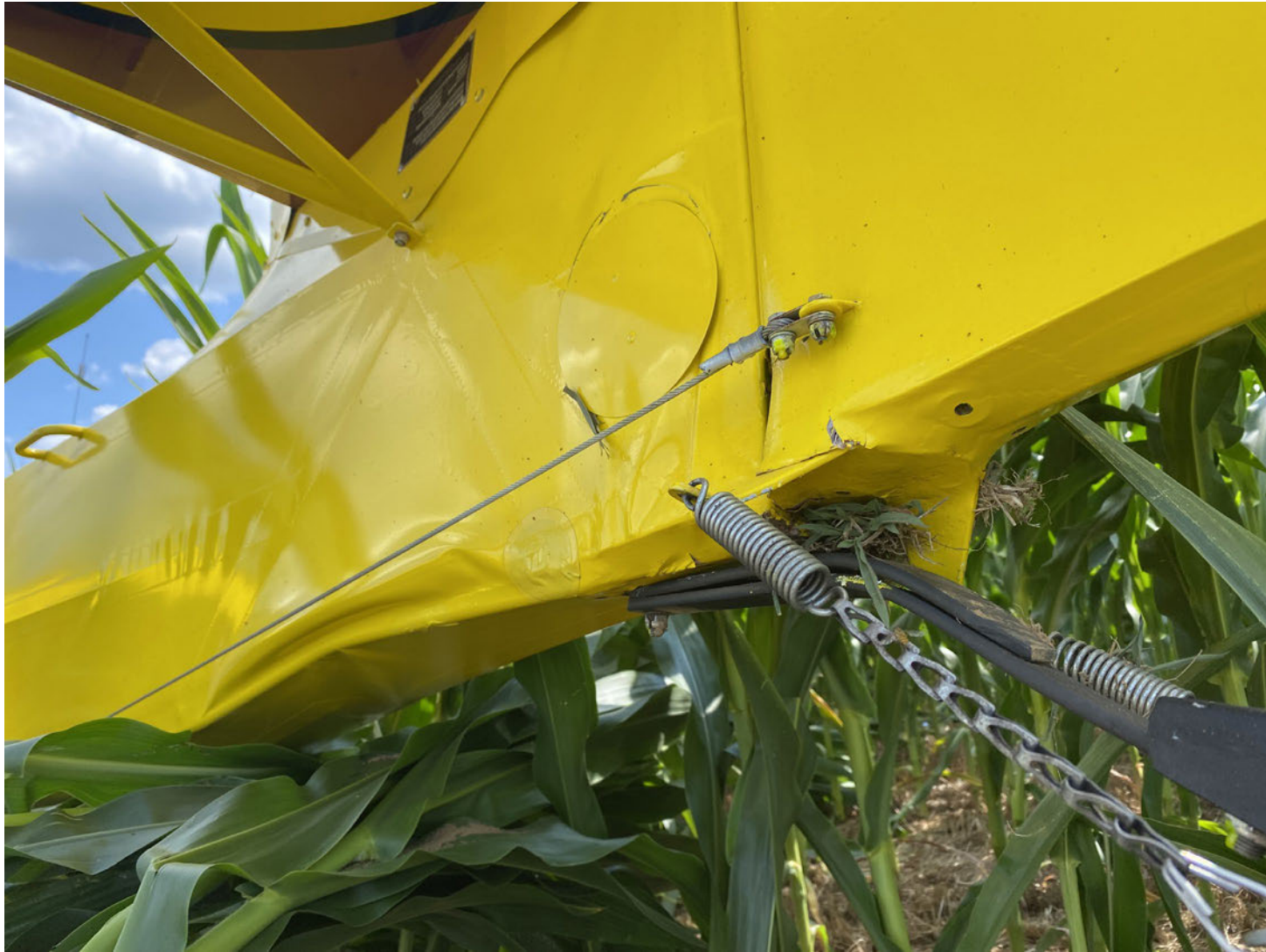
Photograph 2 - Damaged empennage (Courtesy of FAA)
